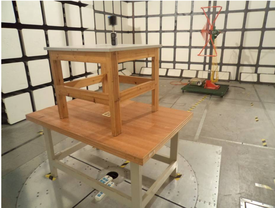
Transmitting Radiated Emissions (Below 1 GHz)
