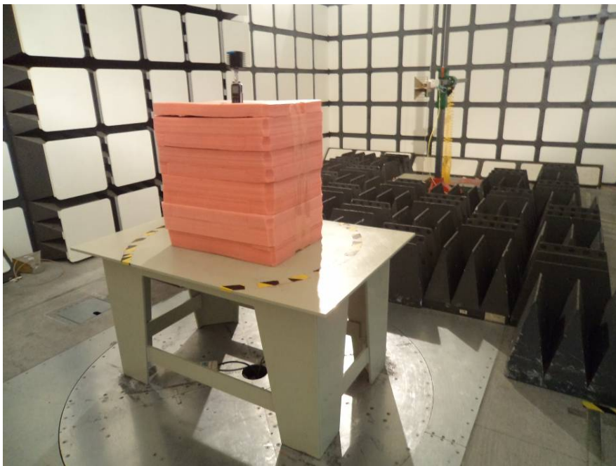
Transmitting Radiated Emissions (Above 1 GHz)
