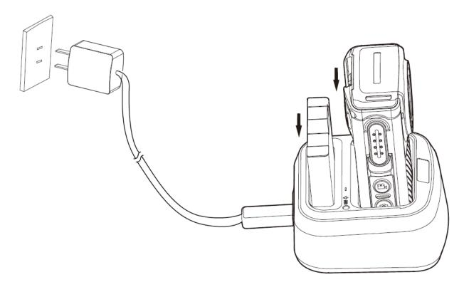
Through the charger, you can charge the product attached with battery and a single battery simultaneously.
