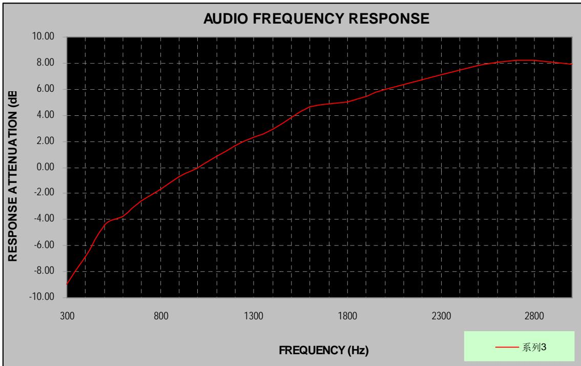
Carrier Frequency: 155.5 MHz, Channel Separation=12.5 kHz, High Power
