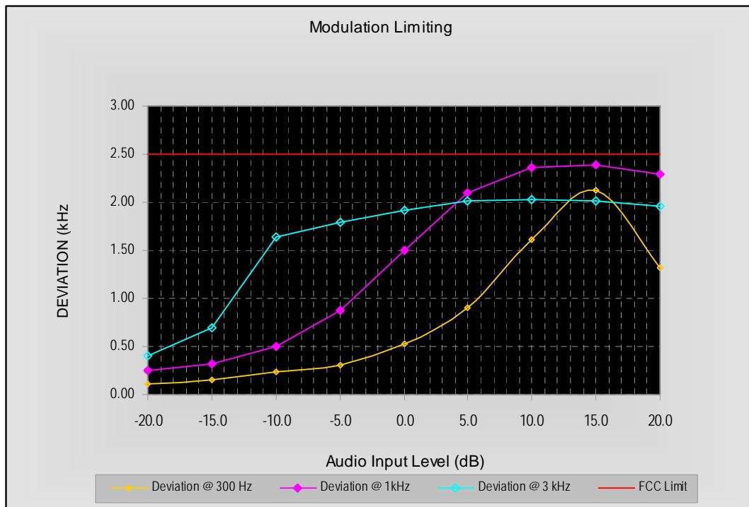
Carrier Frequency: 155.5 MHz, Channel Separation=12.5 kHz, High Power
