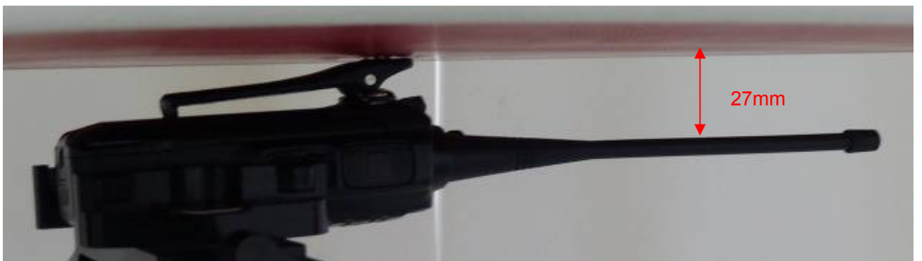
Picture 5: Body-worn, the front of the EUT towards ground, Belt clip directed tightly to touch the bottom of the flat phantom, the distance from the EUT Antenna to the bottom of the Phantom is 27mm
