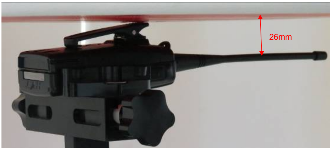
Picture 5: Body-worn, the front of the EUT towards ground, Belt clip directed tightly to touch the bottom of the flat phantom, the distance from the EUT Antenna to the bottom of the Phantom is 26mm
