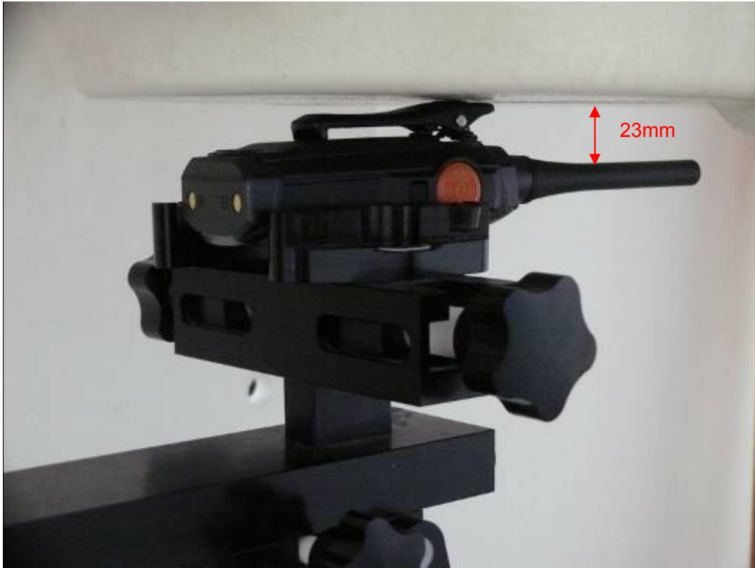
Picture 5: Body-worn, The EUT display towards ground, Belt clip directed tightly to touch the bottom of the flat phantom, the distance from EUT Antenna to the bottom of the Phantom is 23mm
