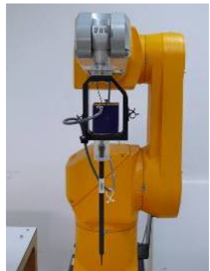
Figure 3. EX3DV4 E-field probe
