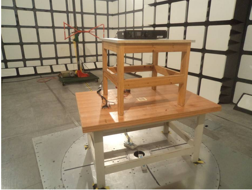
Below 1 GHz: Transmitting Radiated Emissions – Front View
