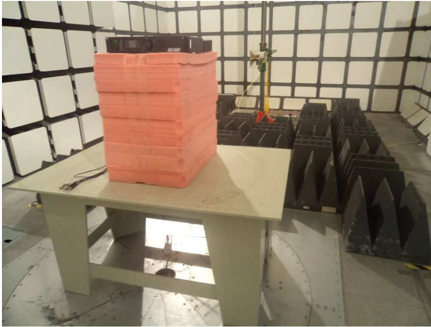
Above 1 GHz: Transmitting Radiated Emissions – Front View
