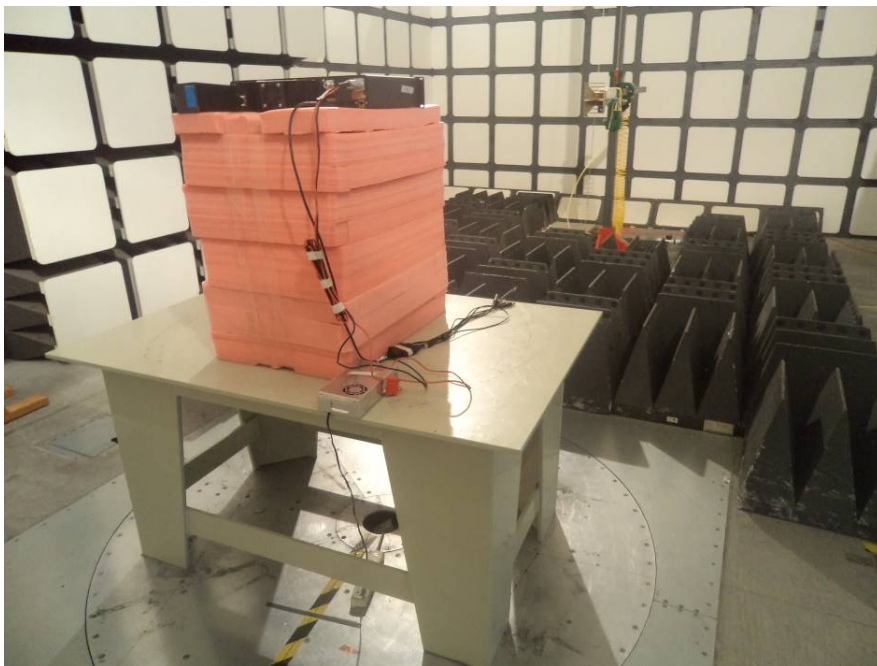
Above 1 GHz: Transmitting Radiated Emissions – Rear View
