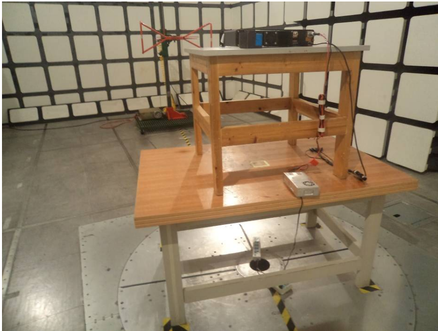
Below 1 GHz: Transmitting Radiated Emissions – Rear View
