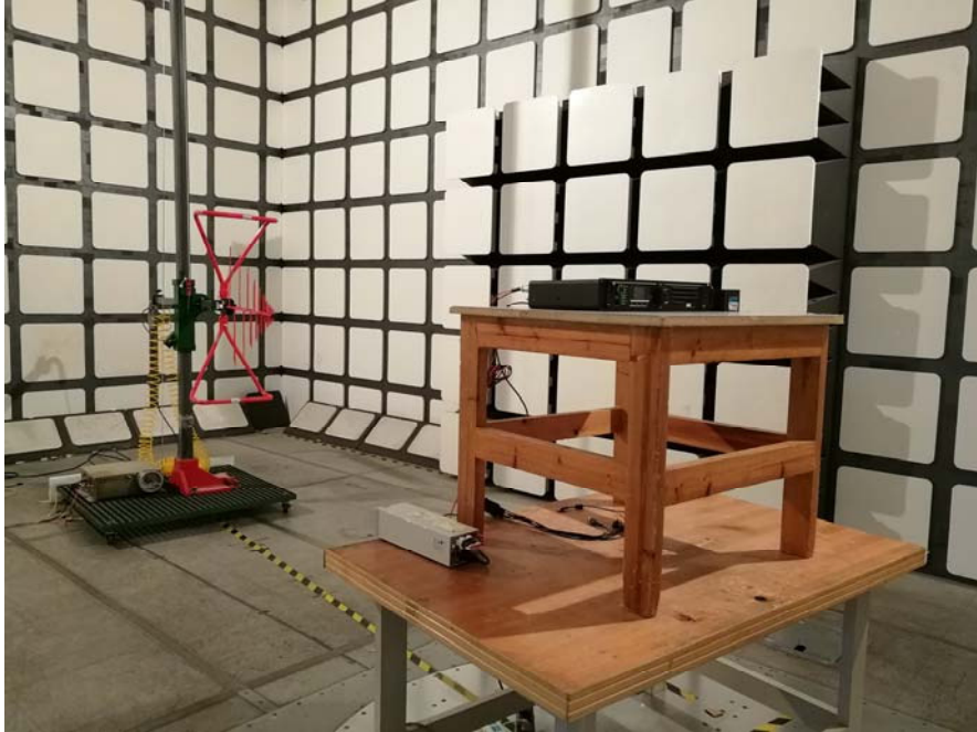
Transmitting Radiated Emissions Tested View (Below 1 GHz)
