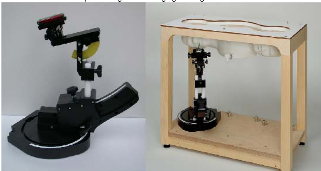
Device holder supplied by SPEAG
