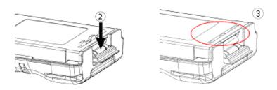
**Step 3** Push the battery as shown below until it is fully fitted into the slot, and then release the battery latch.
