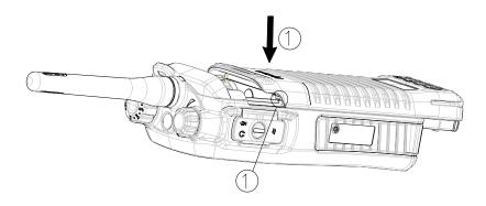
**Step 2** Open the battery latch and exert force on it to retract the metal lock into the battery housing completely as shown below.
