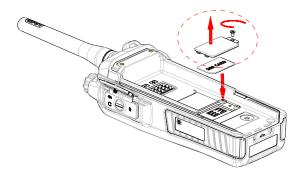
**Step 3** Replace the cover and tighten the screw as shown below.
