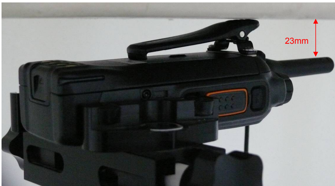
Picture 5: Body-worn with earphone, the front of the EUT towards ground, Belt clip directed tightly to touch the bottom of the flat phantom, the distance from the EUT Antenna to the bottom of the Phantom is 23mm
