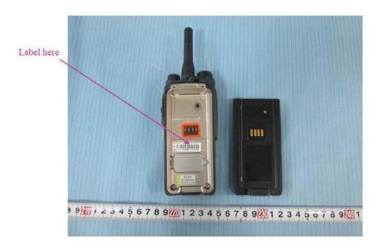
The label shown shall be permanently affixed at a conspicuous location on the device and be readily visible to the user at the time purchase (Labeling requirement per 2.925)
