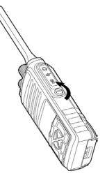
2. Plug the accessory into the accessory connector, and then rotate the screw on the accessory plug clockwise until hand tight.
