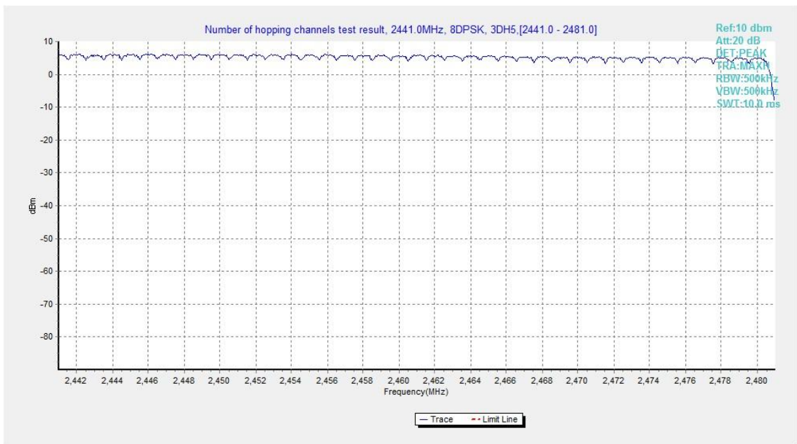
Fig.99. Number of hopping frequencies: 8DPSK, Channel 40 - 78
