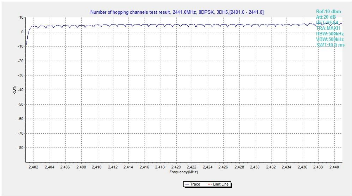
Fig.98. Number of hopping frequencies: 8DPSK, Channel 0 - 39
