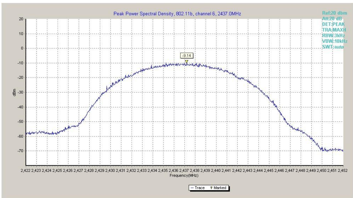
Fig.A.3.2 Power Spectral Density (802.11b, Ch 6)
