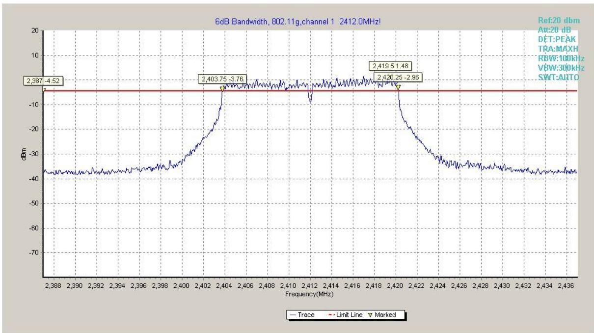
Fig.A.4.4 Occupied 6dB Bandwidth (802.11g, Ch 1)
