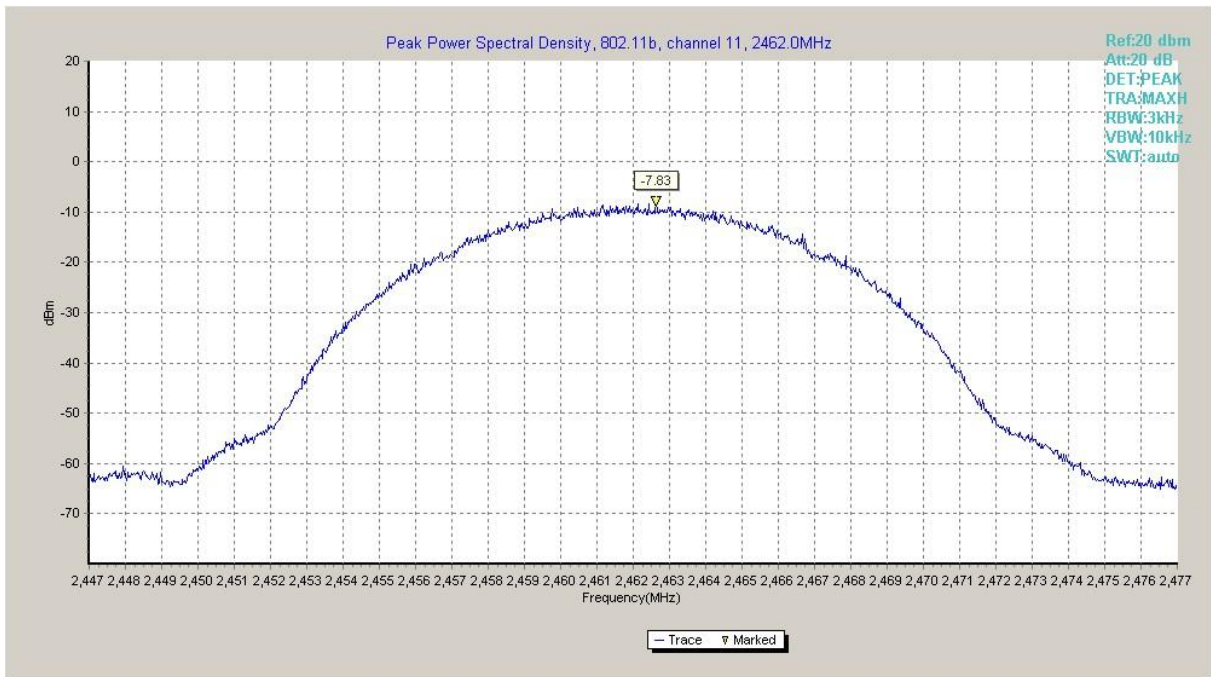
Fig.A.3.3 Power Spectral Density (802.11b, Ch 11)
