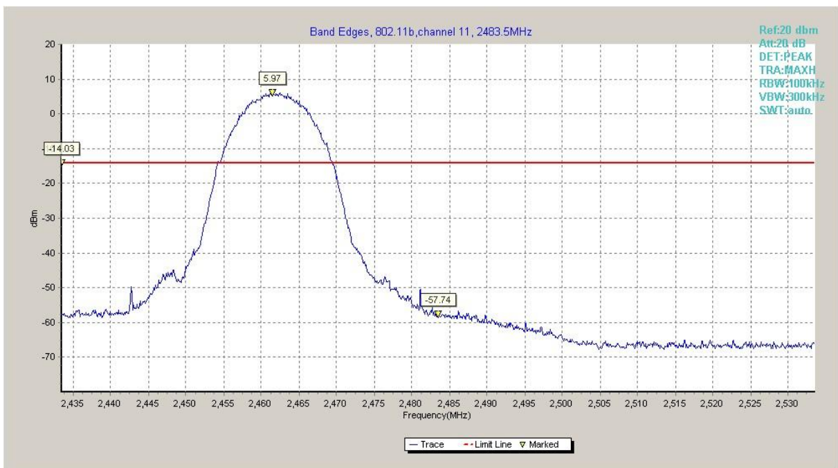
Fig.A.5.2 Band Edges (802.11b, Ch 11)
