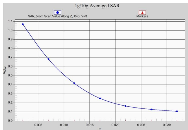
Fig.A.1- 3 Z-Scan at power reference point (PCS1900)
