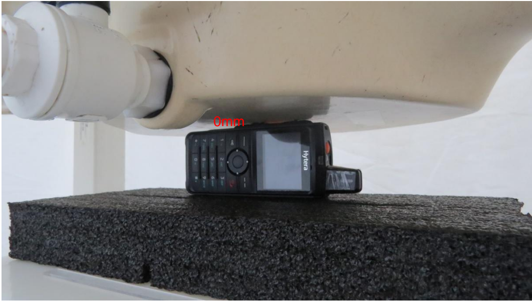
Picture 5: Left Side, the distance from handset to the bottom of the Phantom is 0mm
