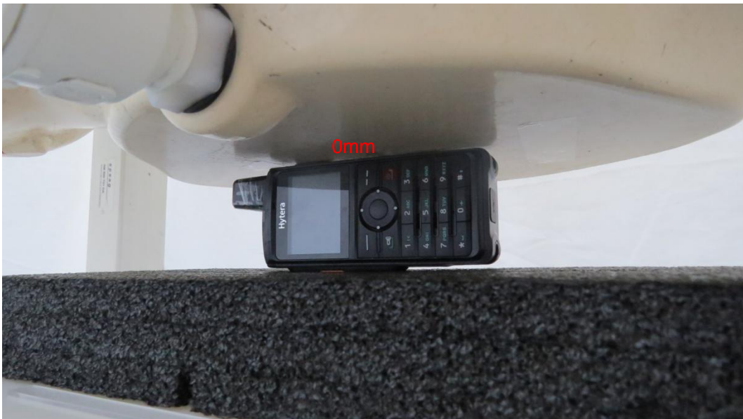
Picture 6: Right Side, the distance from handset to the bottom of the Phantom is 0mm
