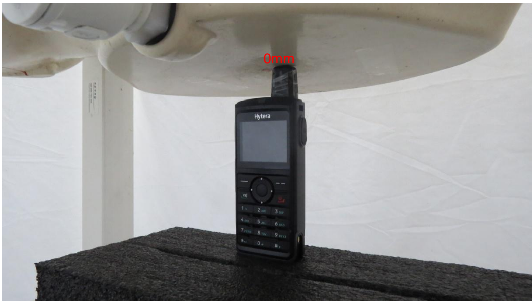
Picture 7: Top Side, the distance from handset to the bottom of the Phantom is 0mm
