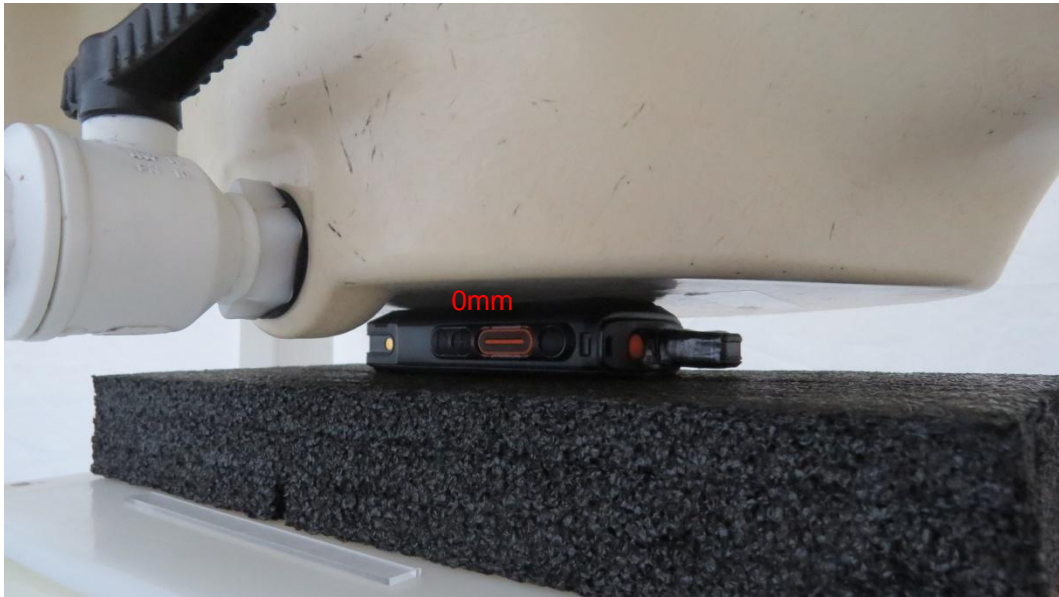
Picture 3: Back Side, the distance from handset to the bottom of the Phantom is 0mm
