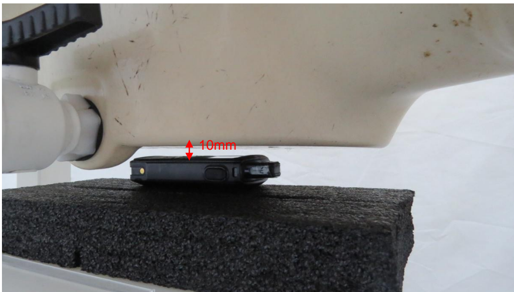
Picture 1: Front Side, the distance from handset to the bottom of the Phantom is 10mm
