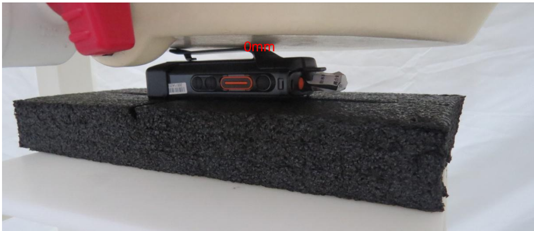
Picture 4: Back Side, the distance from handset to the bottom of the Phantom is 0mm(Body-worn)
