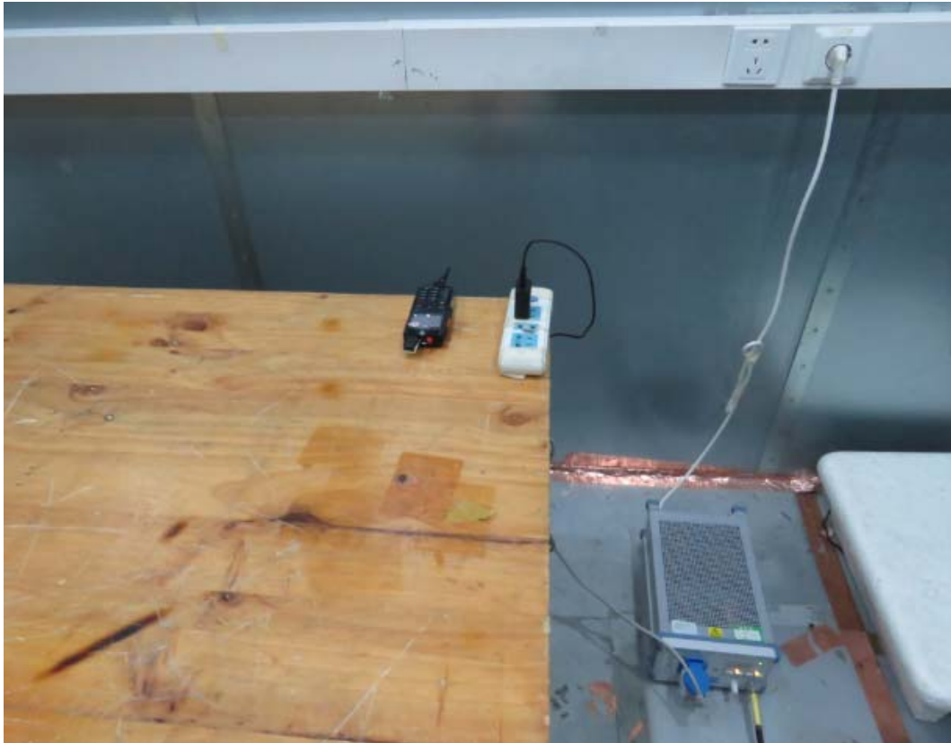
Picture 2 Conducted Emission Test Setup
