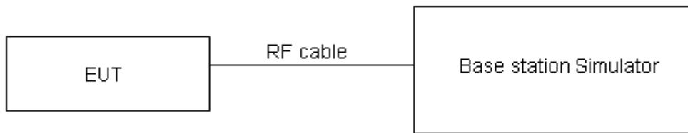
The loss between RF output port of the EUT and the input port of the tester has been taken into consideration.
