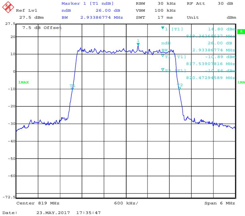
**16-QAM (3.0 MHz) - 26 dB Emissions Bandwidth, Middle channel**
