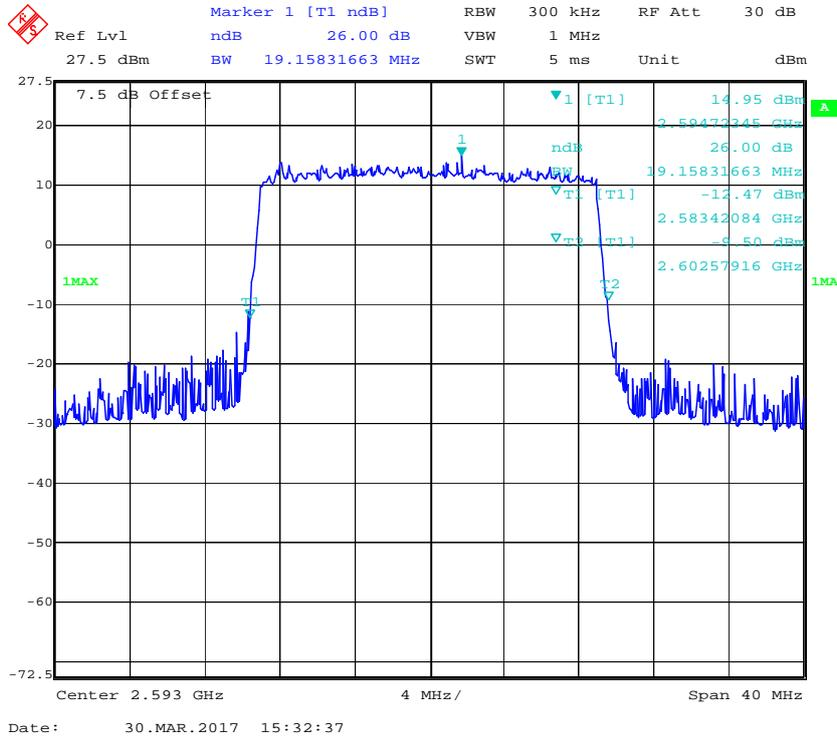
**16-QAM (20.0 MHz) - 26 dB Emissions Bandwidth, Middle channel**
