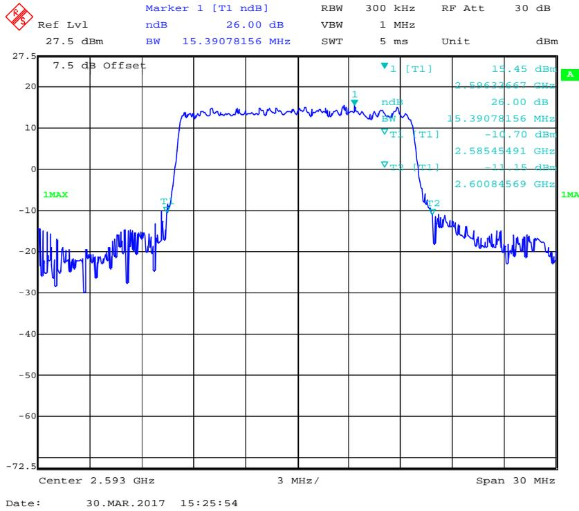
**16-QAM (15.0 MHz) - 26 dB Emissions Bandwidth, Middle channel**
