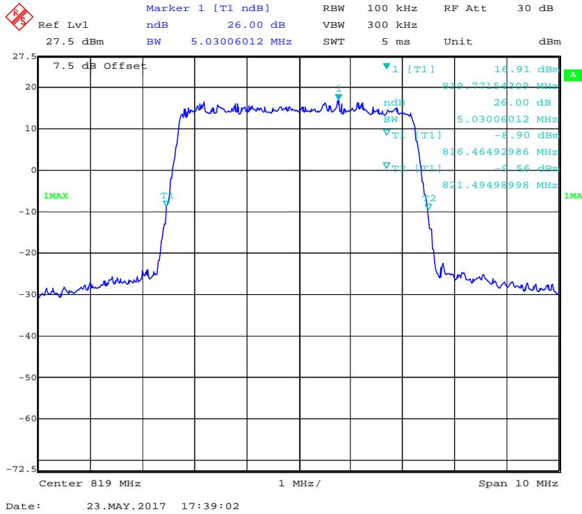
**16-QAM (5.0 MHz) - 26 dB Emissions Bandwidth, Middle channel**
