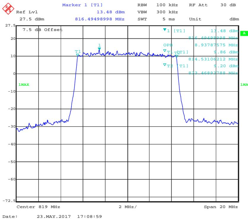
**QPSK (1.4 MHz) - 26 dB Emissions Bandwidth, Middle channel**
