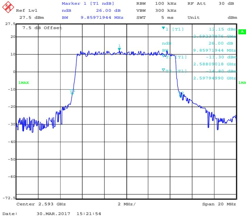
**16-QAM (10.0 MHz) - 26 dB Emissions Bandwidth, Middle channel**
