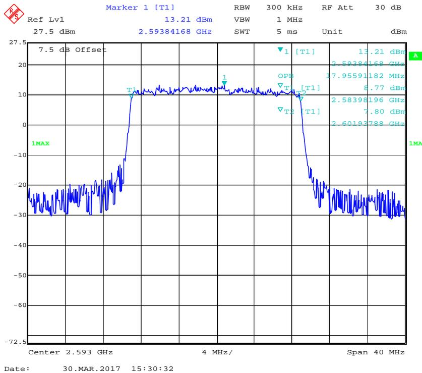
**QPSK (5.0 MHz) - 26 dB Emissions Bandwidth, Middle channel**
