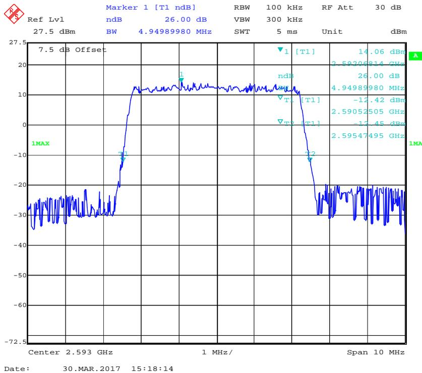
**QPSK (10.0 MHz) - 26 dB Emissions Bandwidth, Middle channel**
