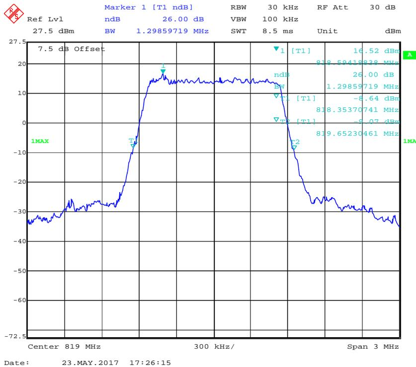
**QPSK (3.0 MHz) - 26 dB Emissions Bandwidth, Middle channel**
