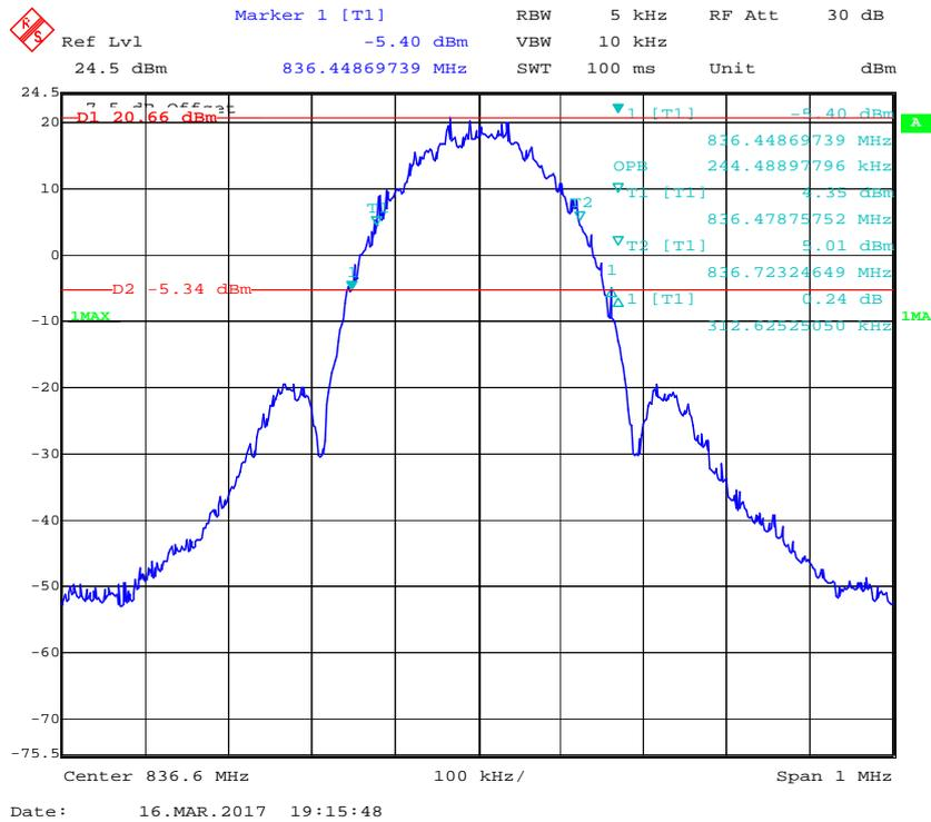
26 dB Emissions & 99% Occupied Bandwidth for CDMA Mode, Middle channel
