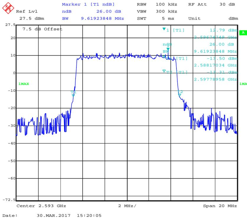
**QPSK (15.0 MHz) - 26 dB Emissions Bandwidth, Middle channel**
