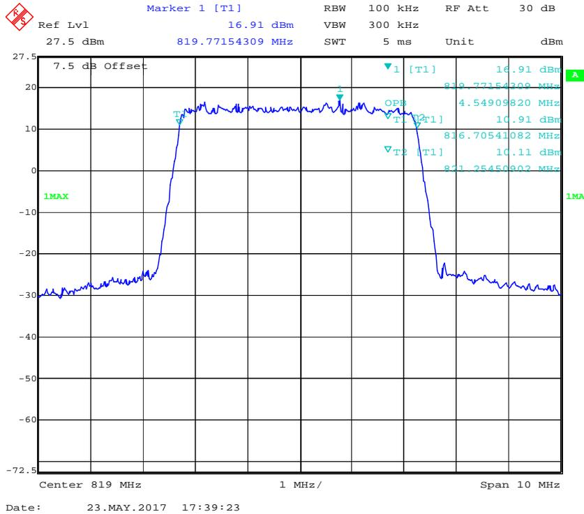
**16-QAM (5.0 MHz) - 99% Occupied Bandwidth, Middle channel**
