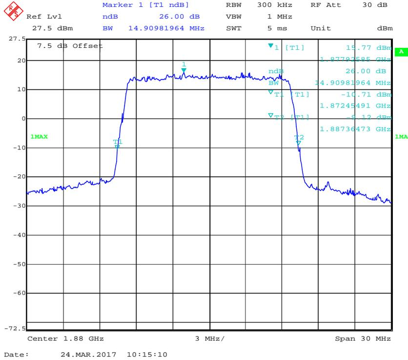
**16-QAM (15.0 MHz) - 26 dB Emissions Bandwidth, Middle channel**
