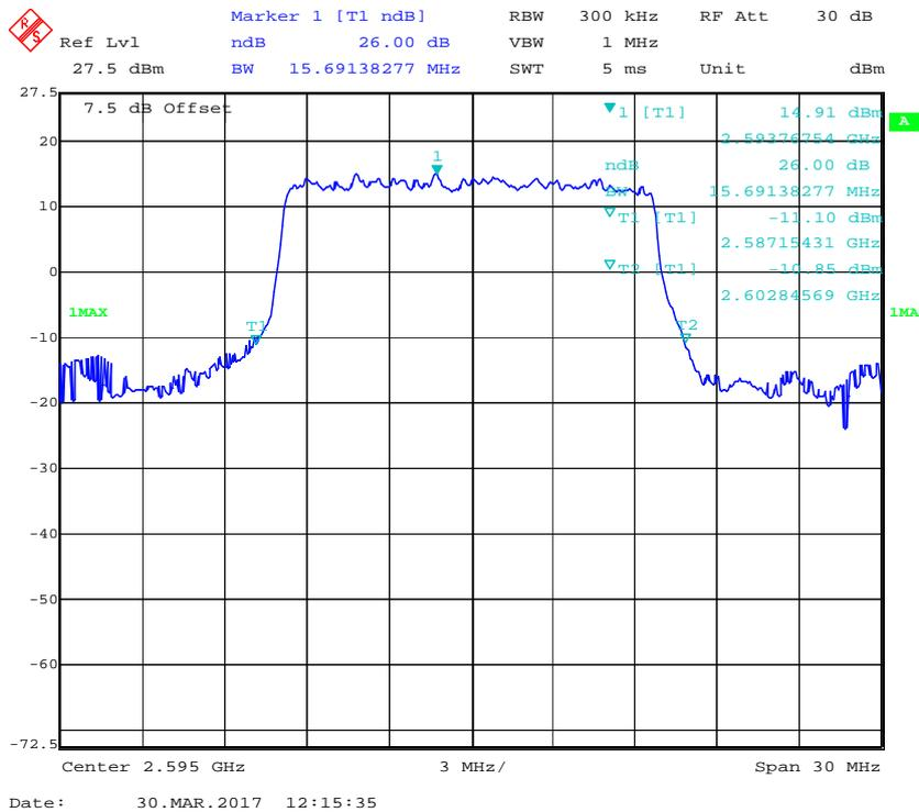
**QPSK (20.0 MHz) - 26 dB Emissions Bandwidth, Middle channel**
