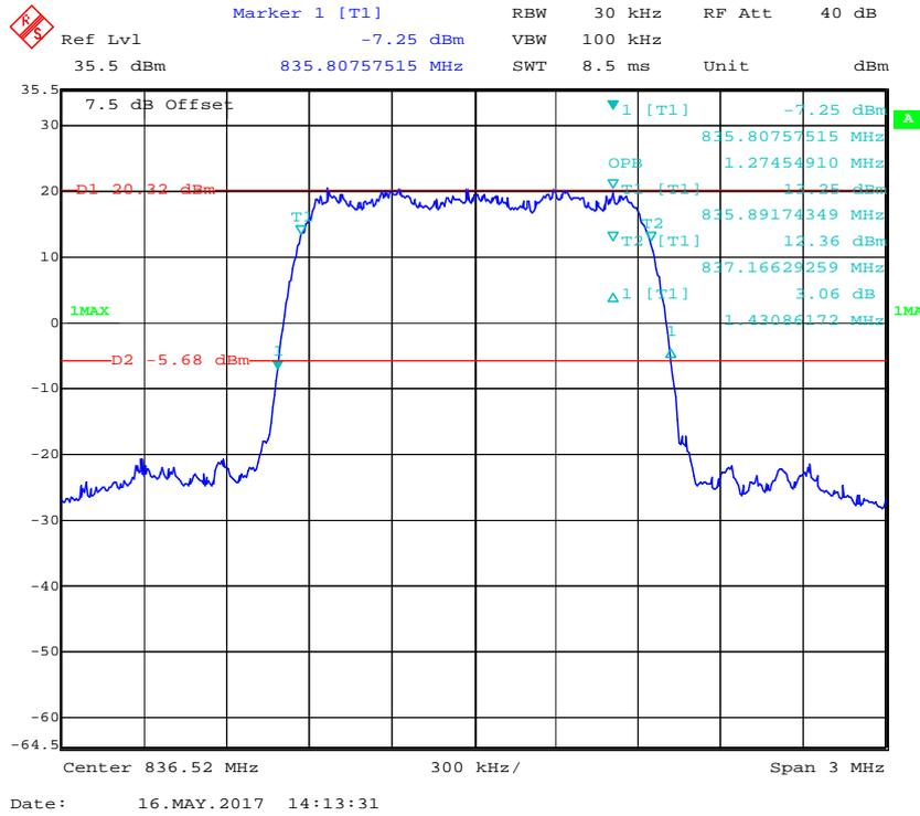
26 dB Emissions & 99% Occupied Bandwidth for CDMA (EV-DO) Mode, Middle channel
