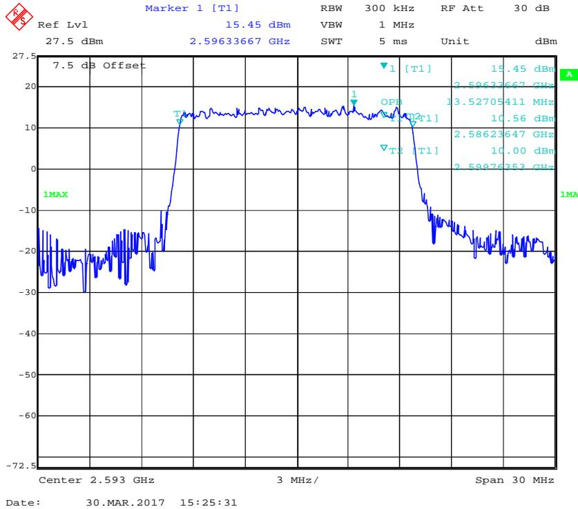
**16-QAM (15.0 MHz) - 99% Occupied Bandwidth, Middle channel**
