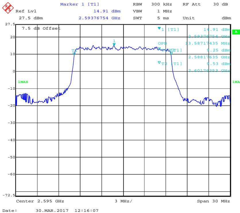
**QPSK (20.0 MHz) - 99% Occupied Bandwidth, Middle channel**
