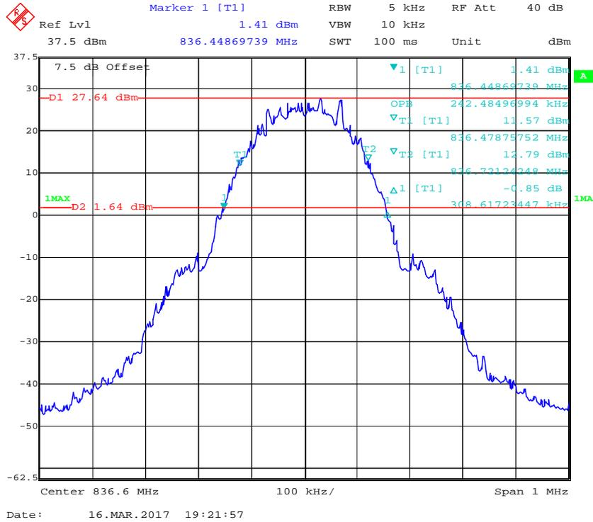
**26 dB Emissions & 99% Occupied Bandwidth for EGPRS (8PSK) Mode**
