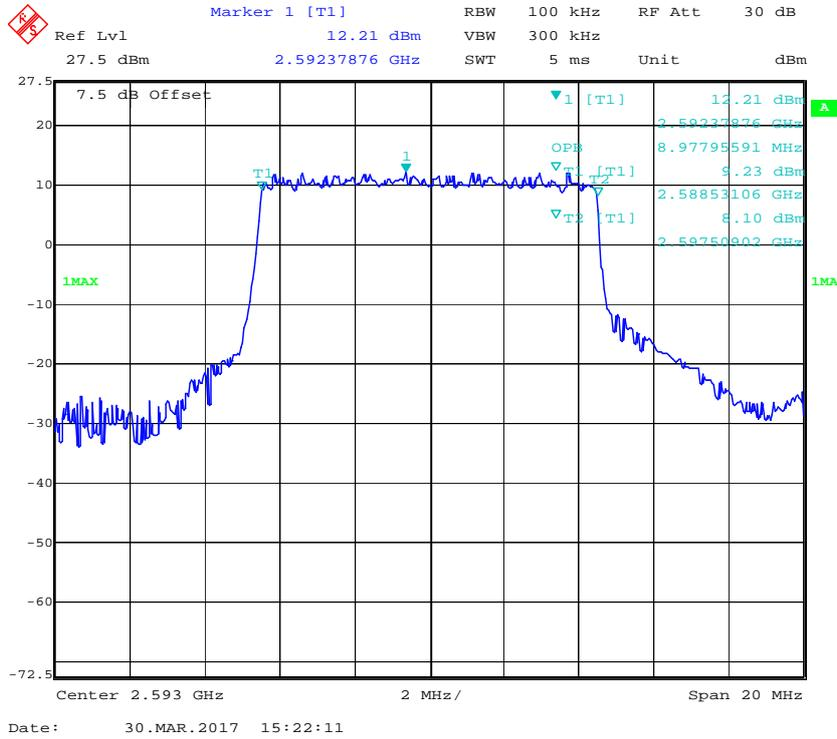
**16-QAM (10.0 MHz) - 99% Occupied Bandwidth, Middle channel**
