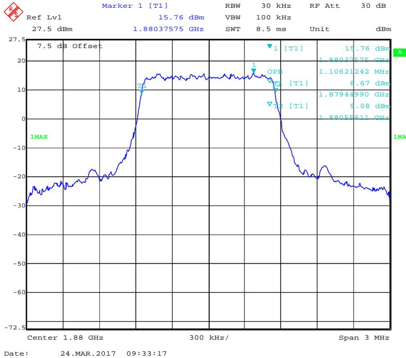
**16-QAM (1.4 MHz) - 99% Occupied Bandwidth, Middle channel**
