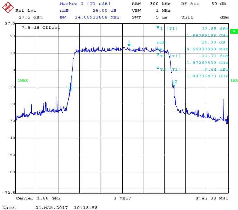
**QPSK (20.0 MHz) - 26 dB Emissions Bandwidth, Middle channel**
