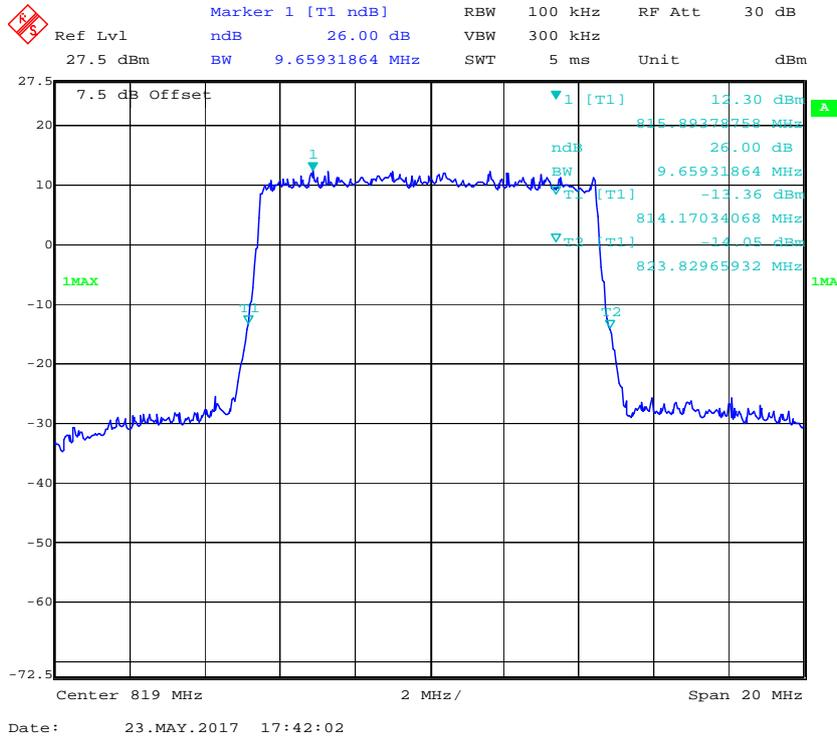
**16-QAM (10.0 MHz) - 26 dB Emissions Bandwidth, Middle channel**
