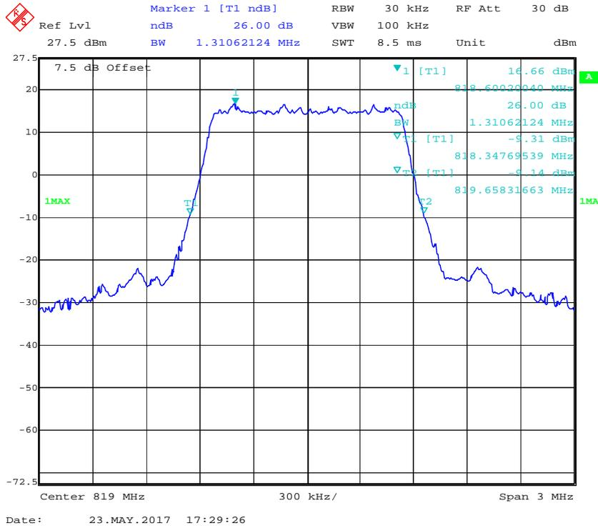
**16-QAM (1.4 MHz) - 26 dB Emissions Bandwidth, Middle channel**
