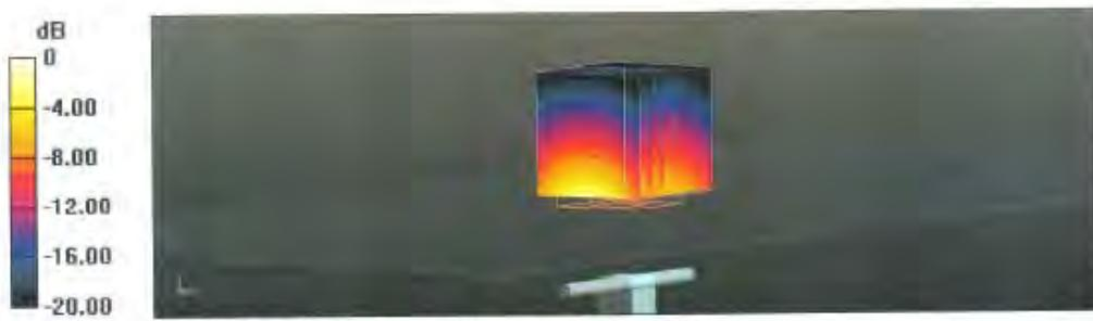
Impedance Measurement Plot for Head TSL
