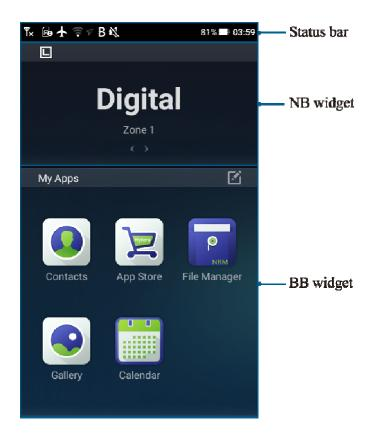
On the main screen, you can also access the notification panel, quick setting panel, and application (app) list. For detailed operations, see 3.4 Operating the Main Screen.
