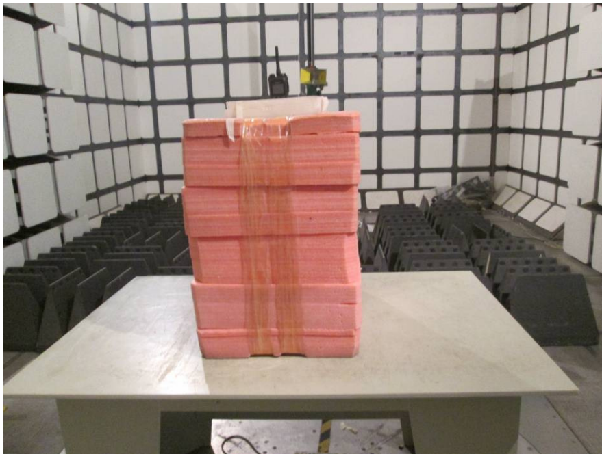
Radiated Emissions Tested View (Above 1GHz)
