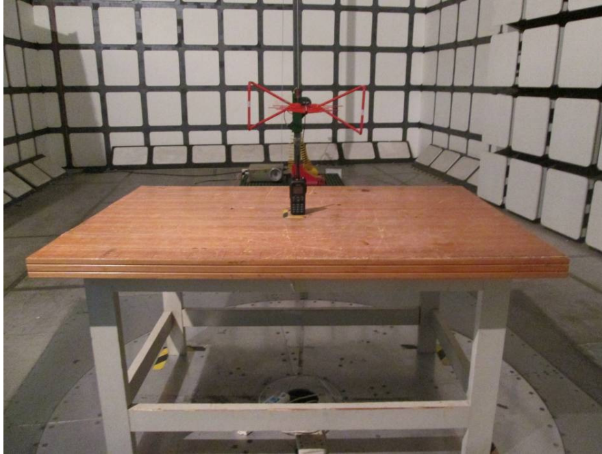
Radiated Emissions Tested View (Below 1GHz)
