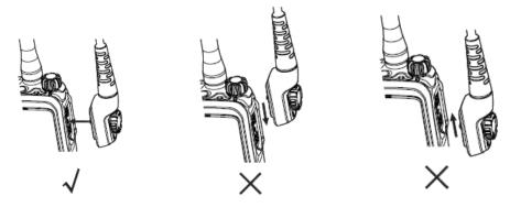
Step 3 Tighten the screw on the accessory plug.
