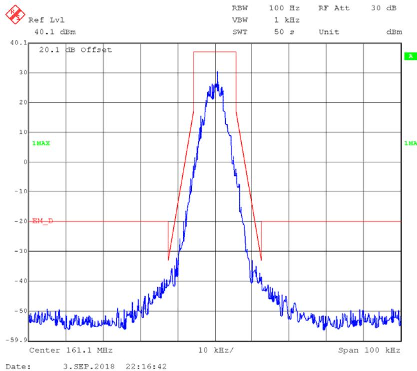
**4FSK,12.5kHz,Low Power - Frequency 161.1 MHz: 99% Occupied & 26 dB Bandwidth**
