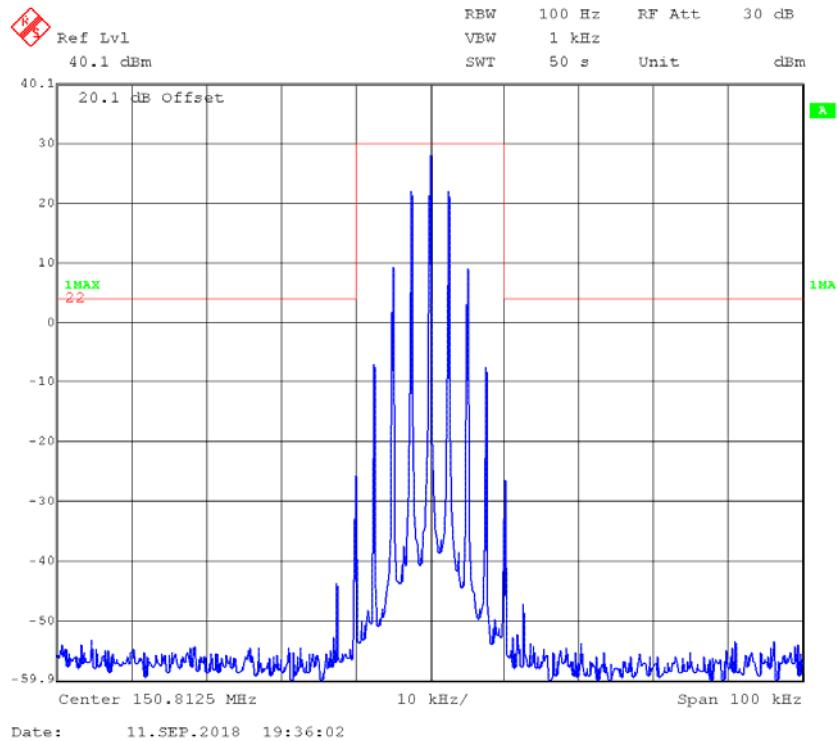
**FM,25kHz,High Power - Frequency 150.8125 MHz: 99% Occupied & 26 dB Bandwidth**
