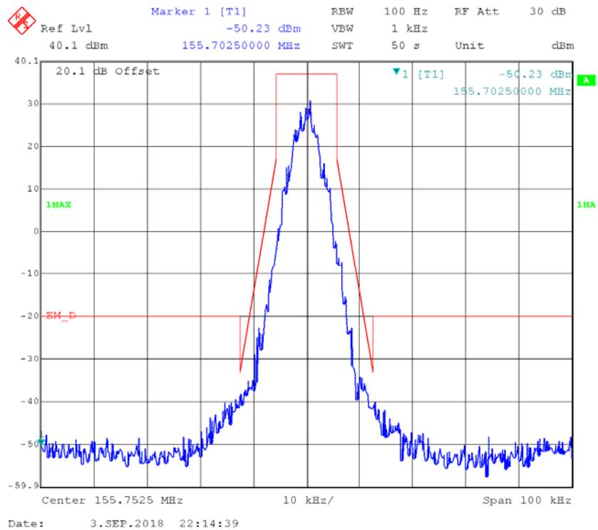
**4FSK,12.5kHz,Low Power - Frequency 155.7525 MHz: 99% Occupied & 26 dB Bandwidth**
