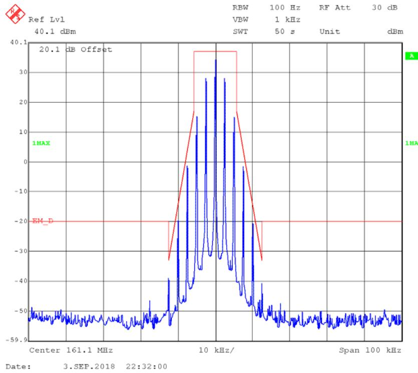
**FM,12.5kHz,Low Power - Frequency 161.1 MHz: 99% Occupied & 26 dB Bandwidth**
