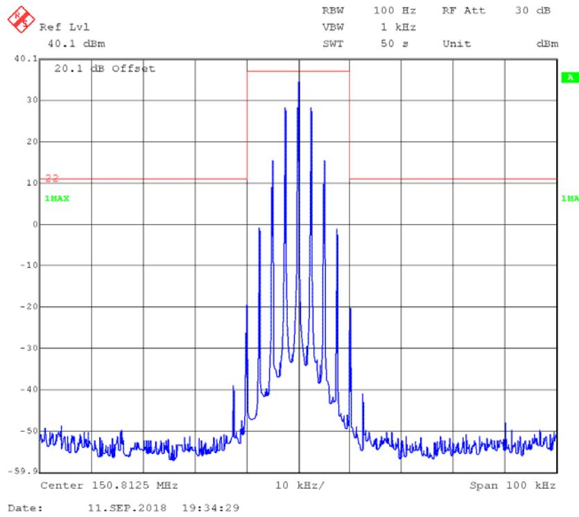
**FM,12.5kHz,Low Power - Frequency 150.8125 MHz: 99% Occupied & 26 dB Bandwidth**
