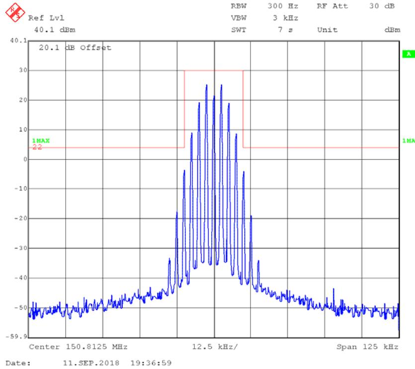
**4FSK,12.5kHz,High Power - Frequency 150.8125 MHz: 99% Occupied & 26 dB Bandwidth**
