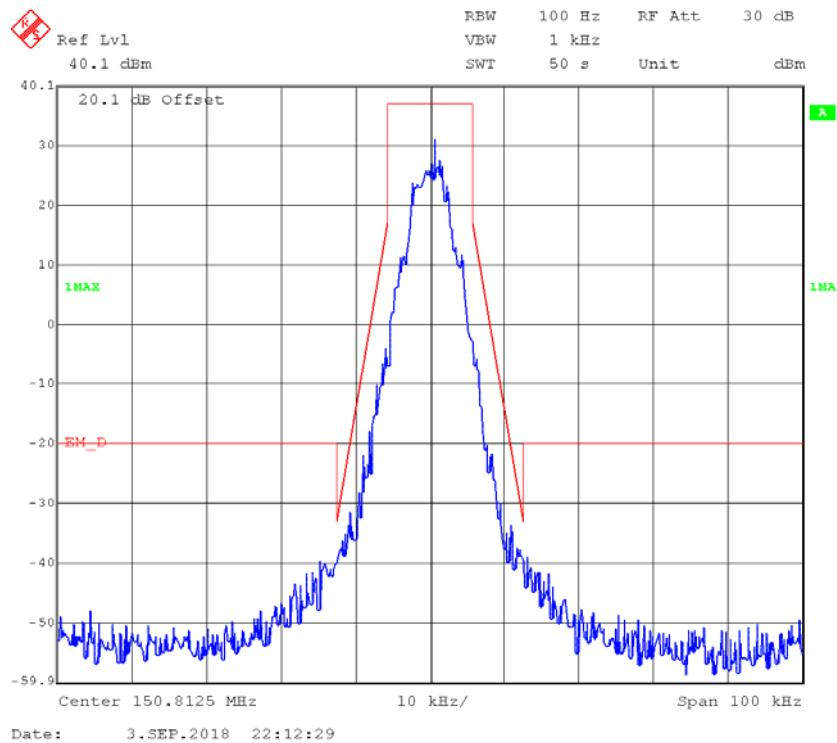
**4FSK,12.5kHz,Low Power - Frequency 150.8125 MHz: 99% Occupied & 26 dB Bandwidth**
