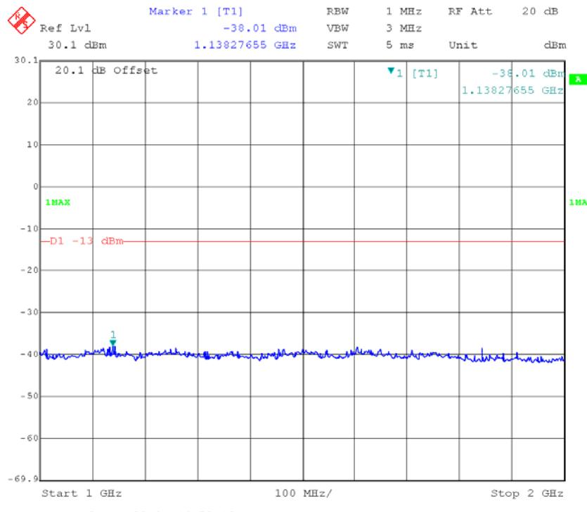
**25kHz,FM, High power:****30MHz – 1 GHz, Channel Spacing 25 kHz, 150.8125 MHz**
