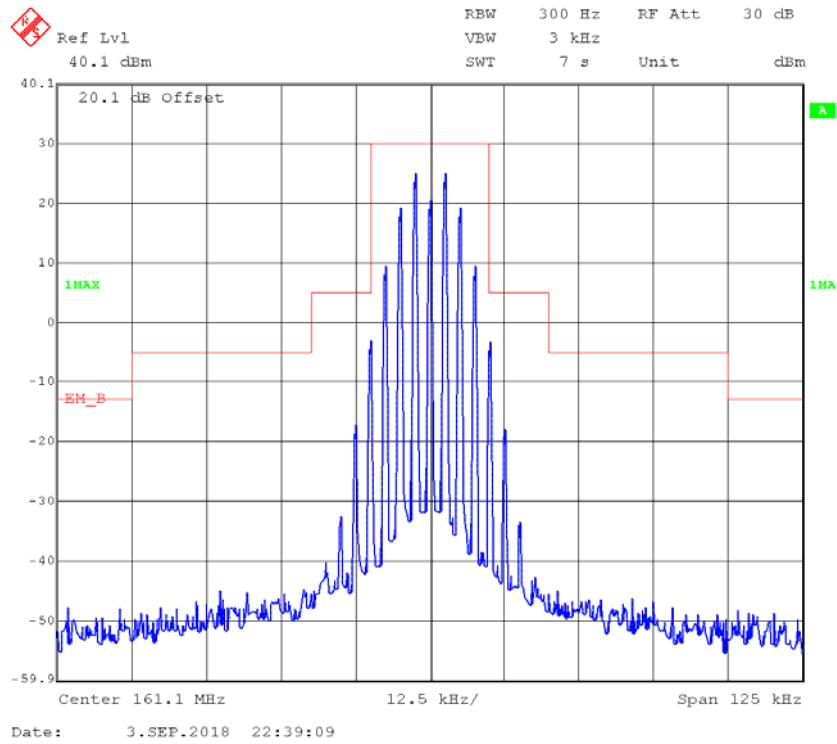
**4FSK,12.5kHz,High Power - Frequency 161.1 MHz: 99% Occupied & 26 dB Bandwidth**
