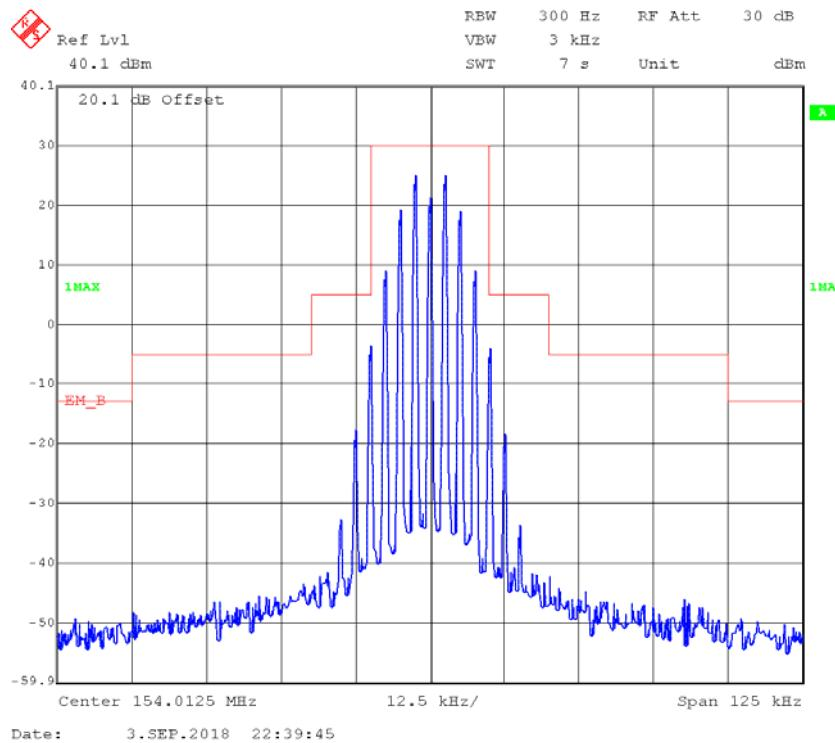
**Part 74****FM,12.5kHz,High Power - Frequency 161.1 MHz: 99% Occupied & 26 dB Bandwidth**
