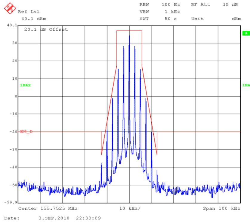
**FM,12.5kHz,Low Power - Frequency 155.7525 MHz: 99% Occupied & 26 dB Bandwidth**
