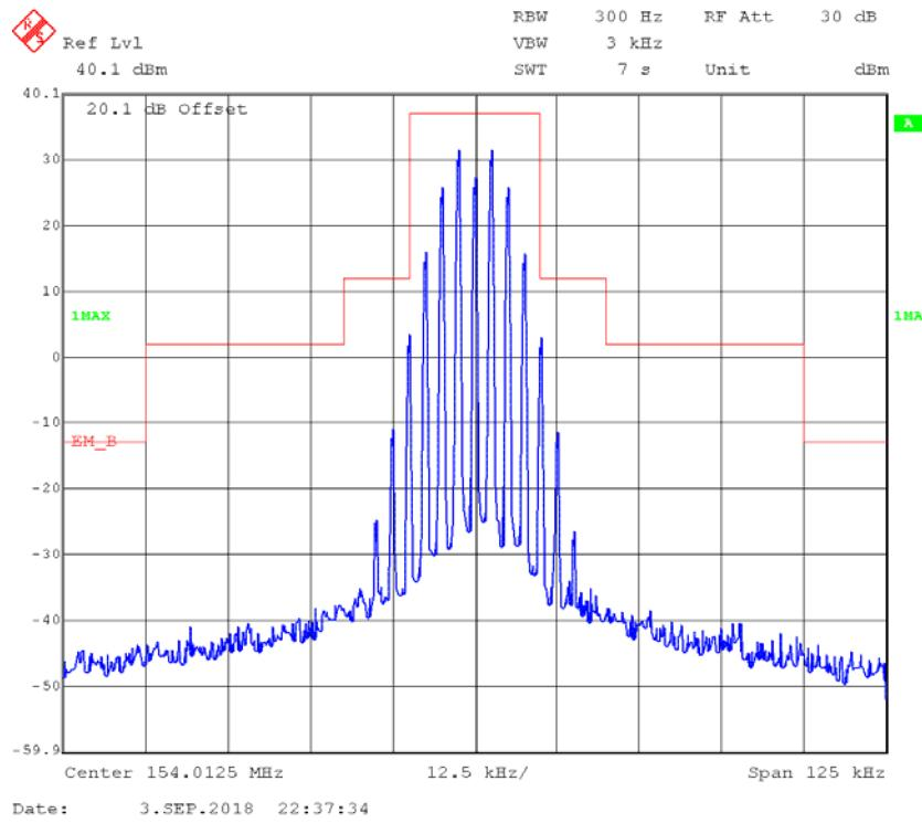
**FM,25kHz,Low Power - Frequency 154.0125 MHz MHz: 99% Occupied & 26 dB Bandwidth**
