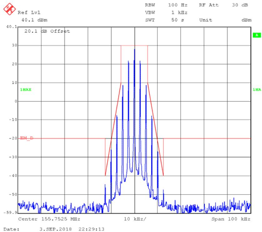
**4FSK,12.5kHz,High Power - Frequency 155.7525 MHz: 99% Occupied & 26 dB Bandwidth**
