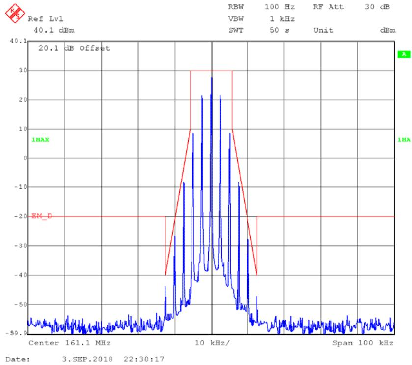
**FM,25kHz,High Power - Frequency 161.1 MHz: 99% Occupied & 26 dB Bandwidth**
