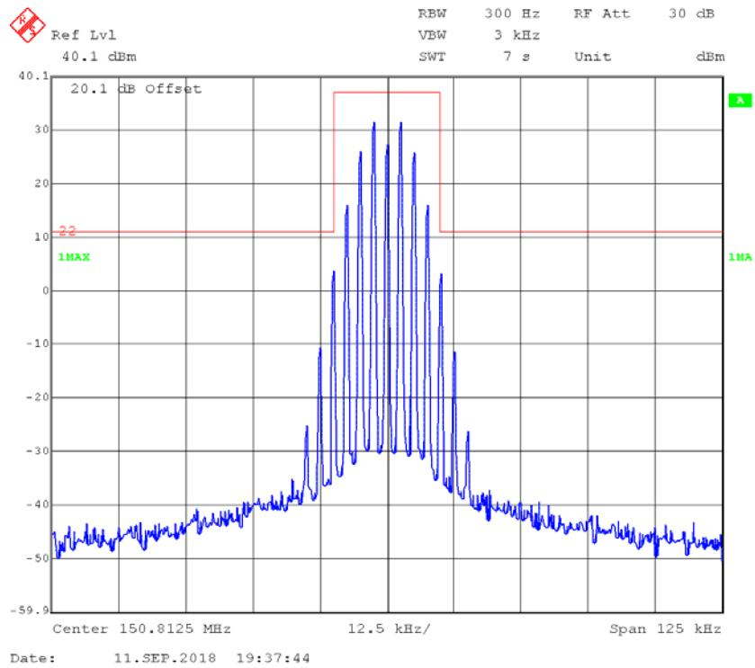
**FM,25kHz,Low Power - Frequency 150.8125 MHz: 99% Occupied & 26 dB Bandwidth**
