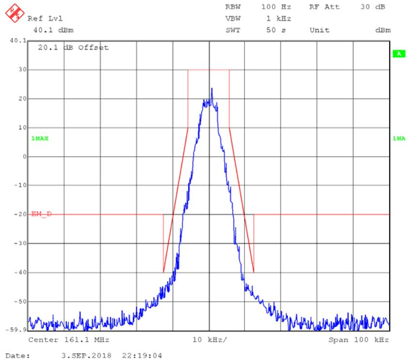
**Part 22****FM,12.5kHz,High Power - Frequency 150.8125 MHz: 99% Occupied & 26 dB Bandwidth**
