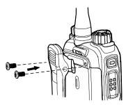
To remove the belt clip, loosen the screws.
