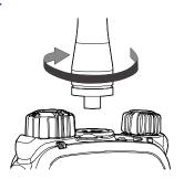
To remove the antenna, rotate it counter-clockwise.
