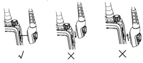
Step 3 Tighten the screw on the connector.
