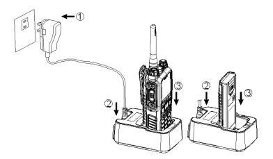
Step 1 Connect the power adapter to AC socket. See arrow ①.
