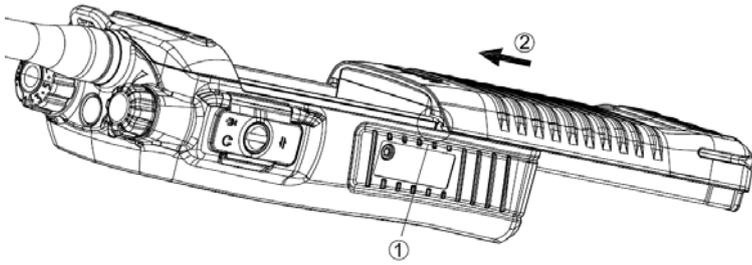
2. Open the battery latch and hold it down until the metal lock goes into the battery housing completely.
