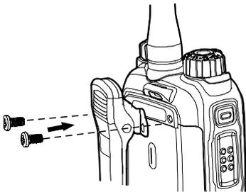
To remove the belt clip, loosen the screws.
