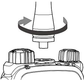
To remove the antenna, rotate it counter-clockwise.
