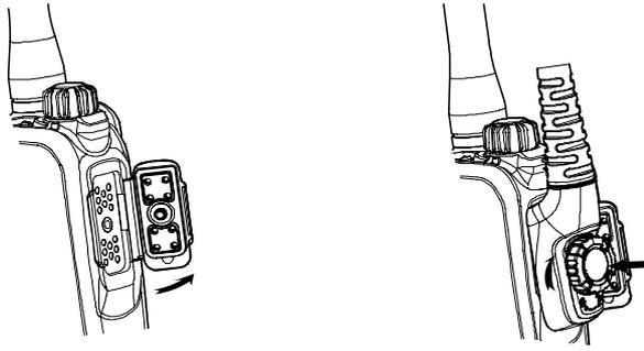
To remove accessories, loosen the screw.
