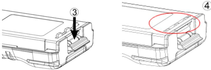
3. Push the battery until it is fully fitted into the slot, and then release the battery latch.
