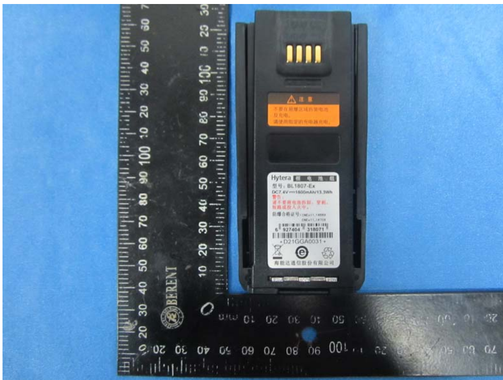
B1- Battery, Intrinsically Safe Li-ion Battery(1800mAh): BL1807-Ex
