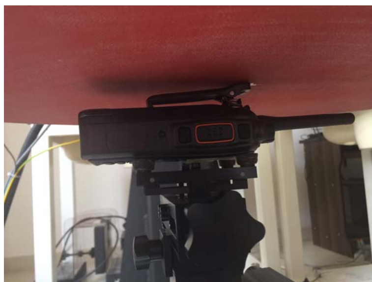
Body-worn, The EUT display towards ground, belt clip attach the phantom
