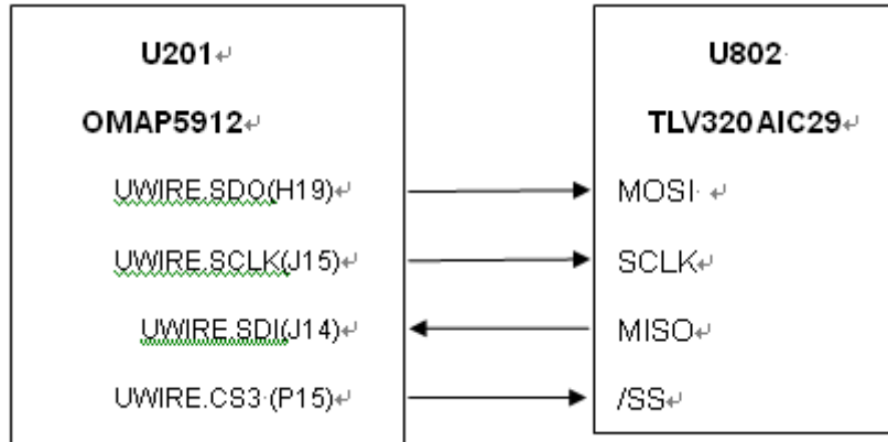
Figure 16 Diagram of MICROWIRE Connection
