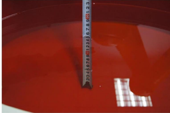
Liquid depth in the flat Phantom (150MHz) (15.3cm deep)
