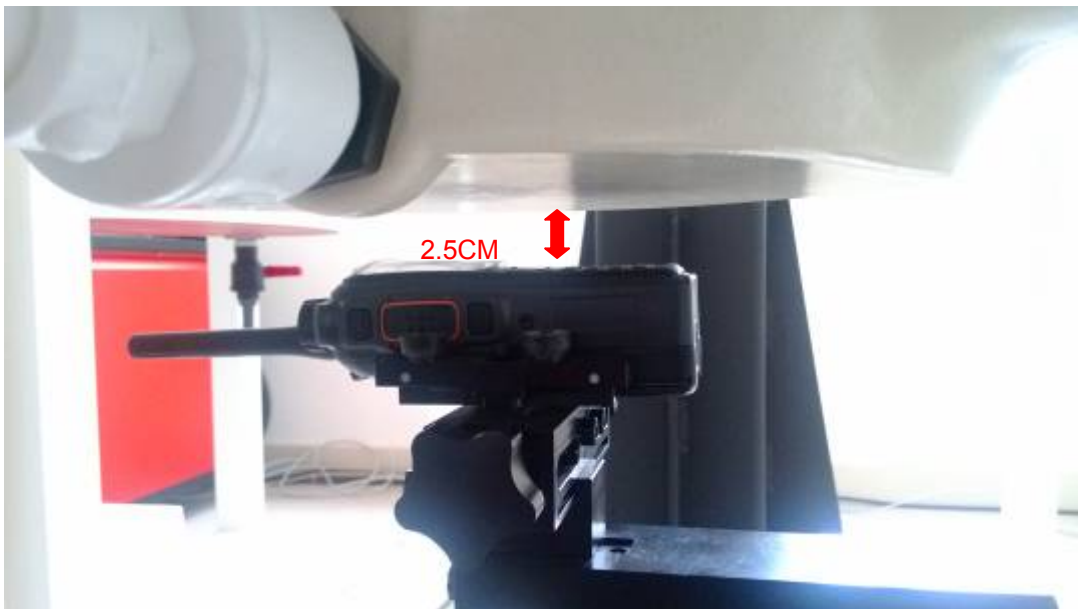
Face-held with Thicker Battery, the front of the EUT towards phantom
