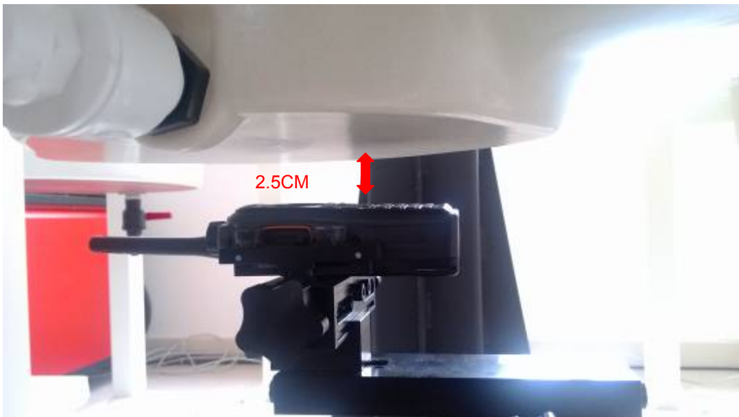
Face-held with Thinner Battery, the front of the EUT towards phantom
