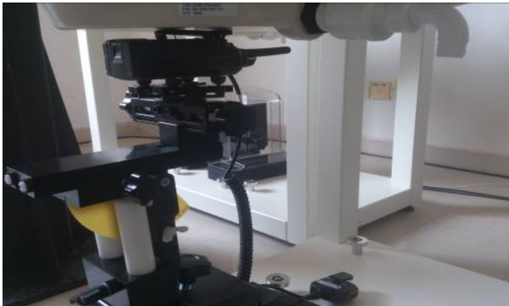
Body-worn with Thicker Battery,Belt, the front of the EUT towards ground
