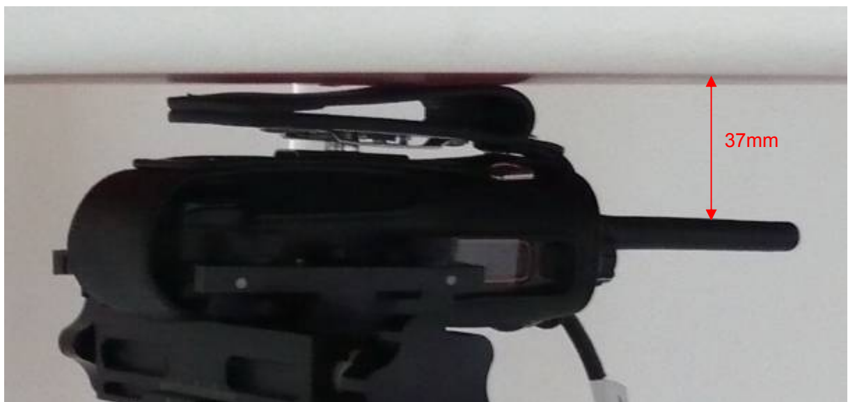
Picture 13: Body-worn with Thinner Battery, Pocket, Leather and Accessory 1, the front of the EUT towards ground, the distance from EUT Antenna to the bottom of the Phantom is 37mm
