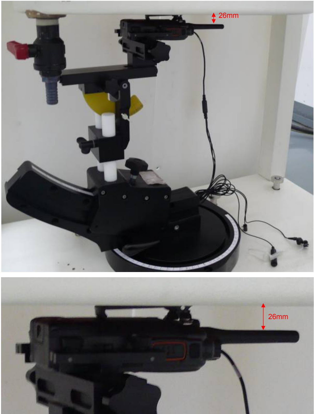
Picture 11: Body-worn with Thinner Battery, Belt and Audio Accessory 4, the front of the EUT towards ground, the distance from EUT Antenna to the bottom of the Phantom is 26mm
