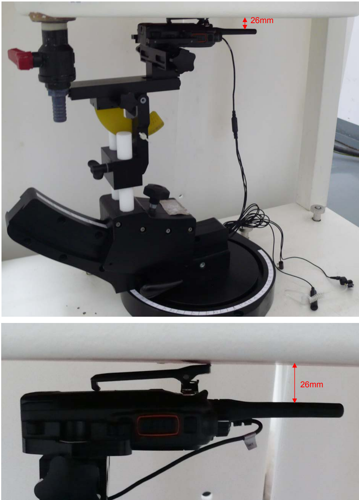
Picture 11: Body-worn with Thinner Battery, Belt and Audio Accessory 4, the front of the EUT towards ground, the distance from EUT Antenna to the bottom of the Phantom is 26mm
