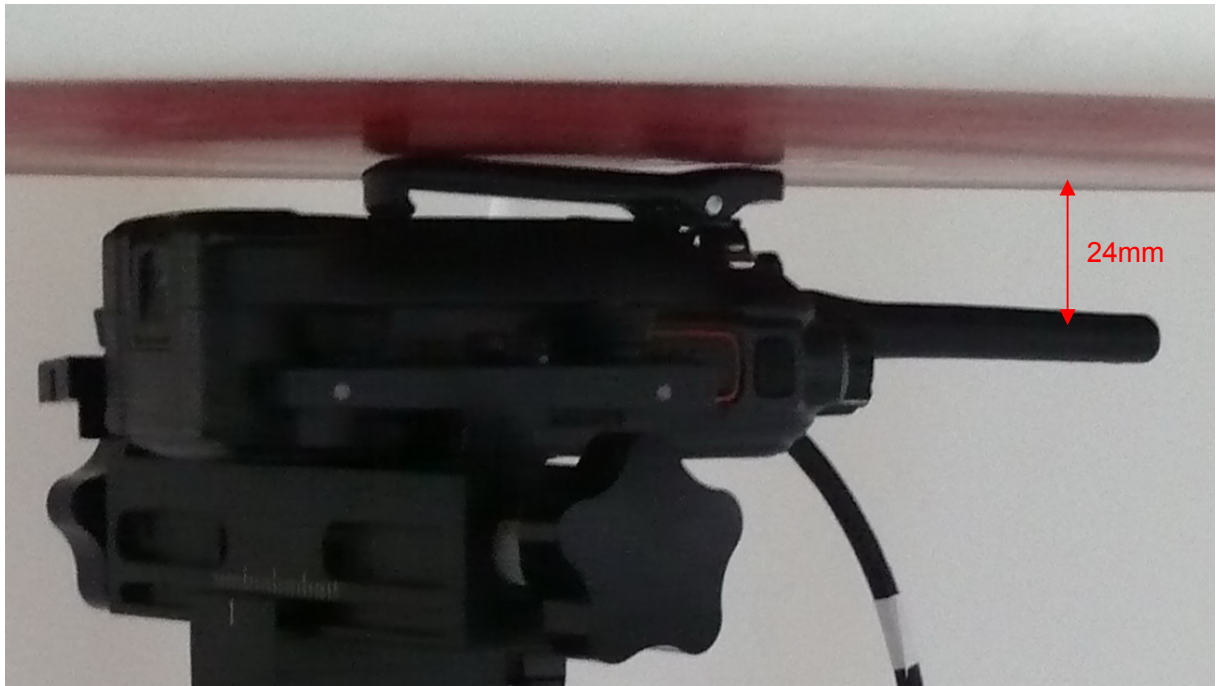
Picture 15: Body-worn with Thicker Battery, Belt and Accessory 1, the front of the EUT towards ground, the distance from EUT Antenna to the bottom of the Phantom is 24mm
