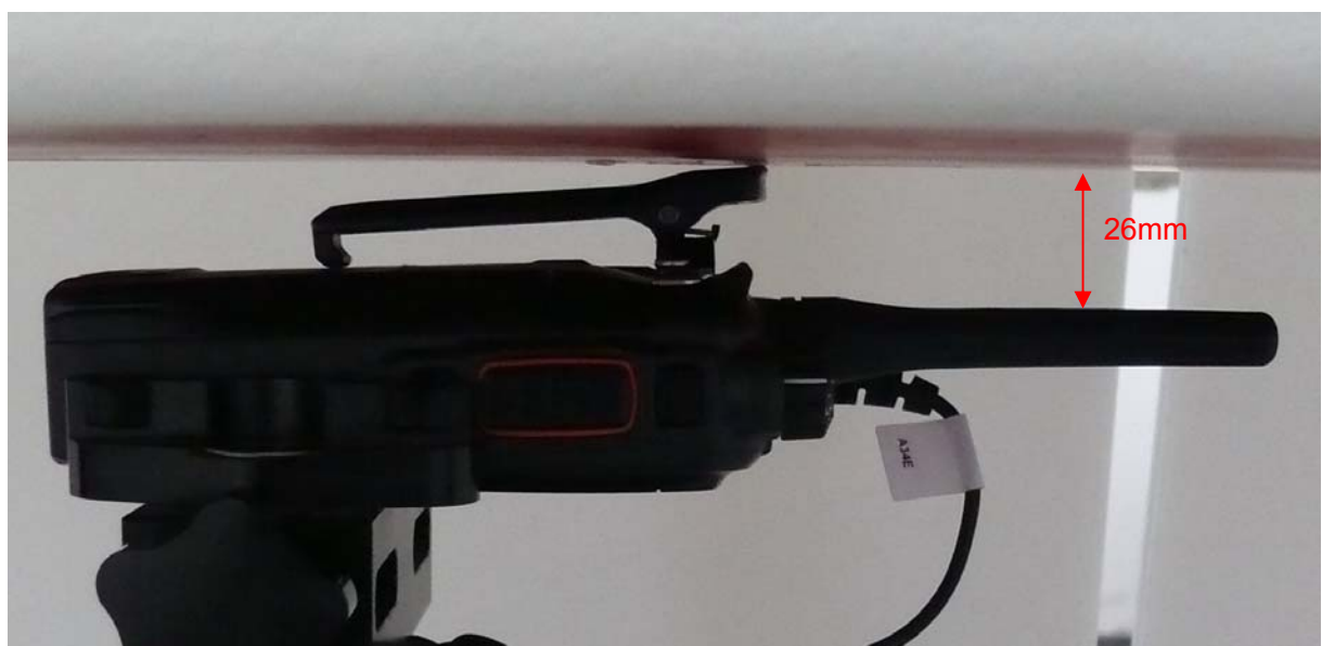
Picture 12: Body-worn with Thinner Battery, Belt and Audio Accessory 5, the front of the EUT towards ground, the distance from EUT Antenna to the bottom of the Phantom is 26mm
