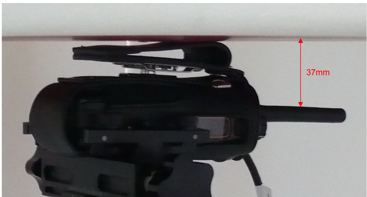
Picture 14: Body-worn with Thinner Battery, Pocket, Leather and Accessory 1, the front of the EUT towards ground, the distance from EUT Antenna to the bottom of the Phantom is 37mm
