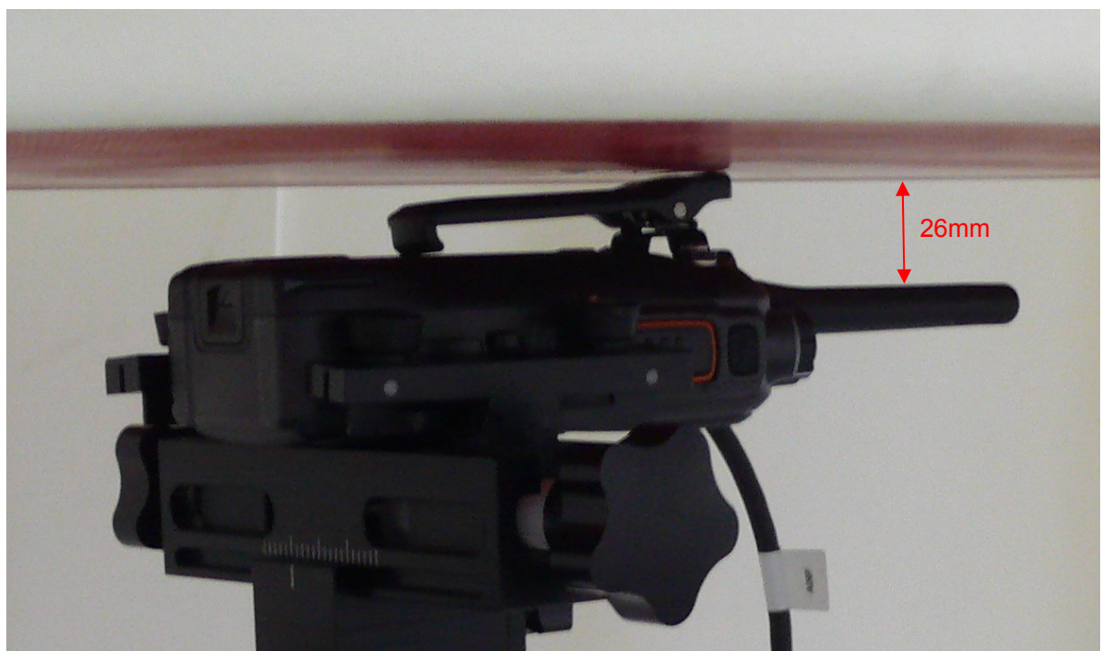
Picture 6: Body-worn with Thinner Battery, Belt and Accessory 1, the front of the EUT towards ground, the distance from EUT Antenna to the bottom of the Phantom is 26mm
