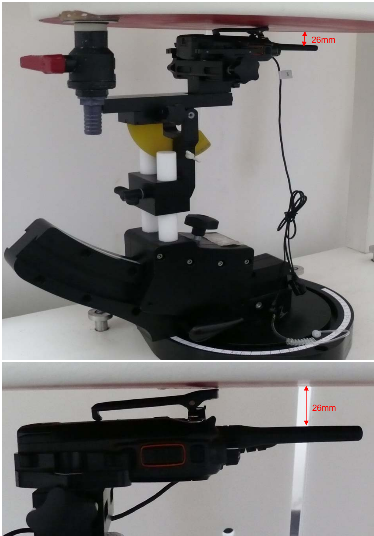
Picture 10: Body-worn with Thinner Battery, Belt and Audio Accessory 3, the front of the EUT towards ground, the distance from EUT Antenna to the bottom of the Phantom is 26mm
