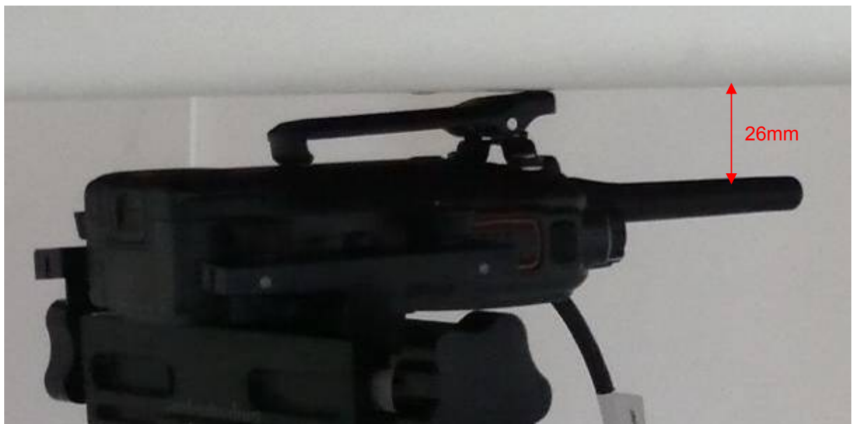
Picture 7: Body-worn with Thinner Battery, Belt, Accessory 1 and Earphone 1, the front of the EUT towards ground, the distance from EUT Antenna to the bottom of the Phantom is 26mm
