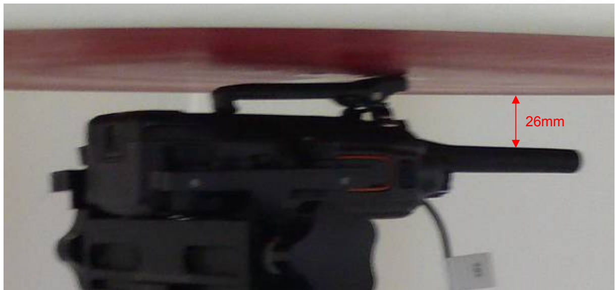
Picture 10: Body-worn with Thinner Battery, Belt and Audio Accessory 3, the front of the EUT towards ground, the distance from EUT Antenna to the bottom of the Phantom is 26mm
