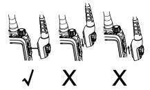
Step 3 Tighten the screw on the plug.
