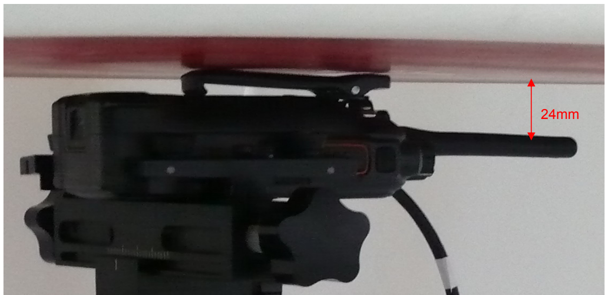
Picture 15: Body-worn with Thicker Battery, Belt and Accessory 1, the front of the EUT towards ground, the distance from EUT Antenna to the bottom of the Phantom is 24mm
