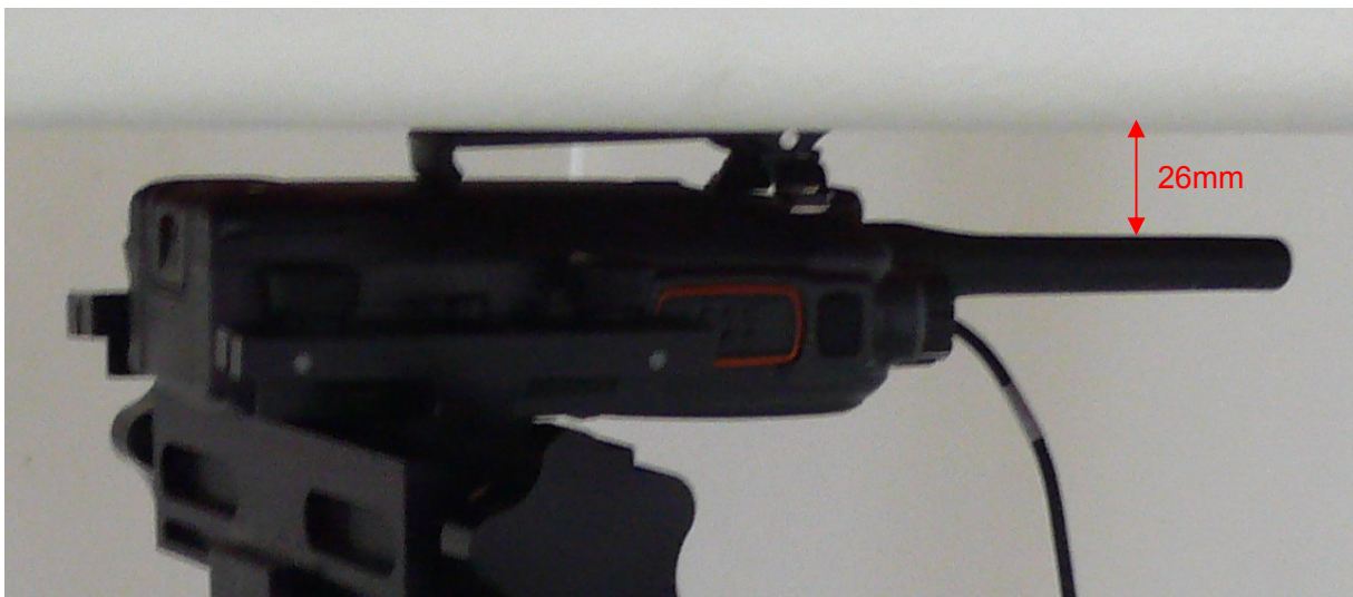
Picture 11: Body-worn with Thinner Battery, Belt and Audio Accessory 4, the front of the EUT towards ground, the distance from EUT Antenna to the bottom of the Phantom is 26mm
