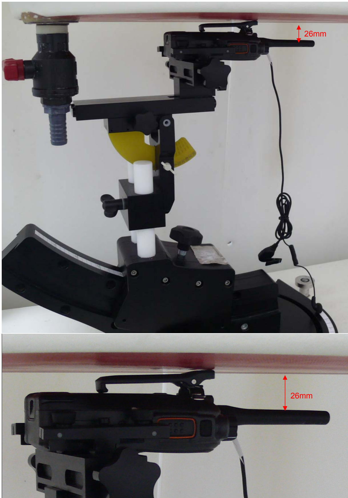
Picture 12: Body-worn with Thinner Battery, Belt and Audio Accessory 5, the front of the EUT towards ground, the distance from EUT Antenna to the bottom of the Phantom is 26mm
