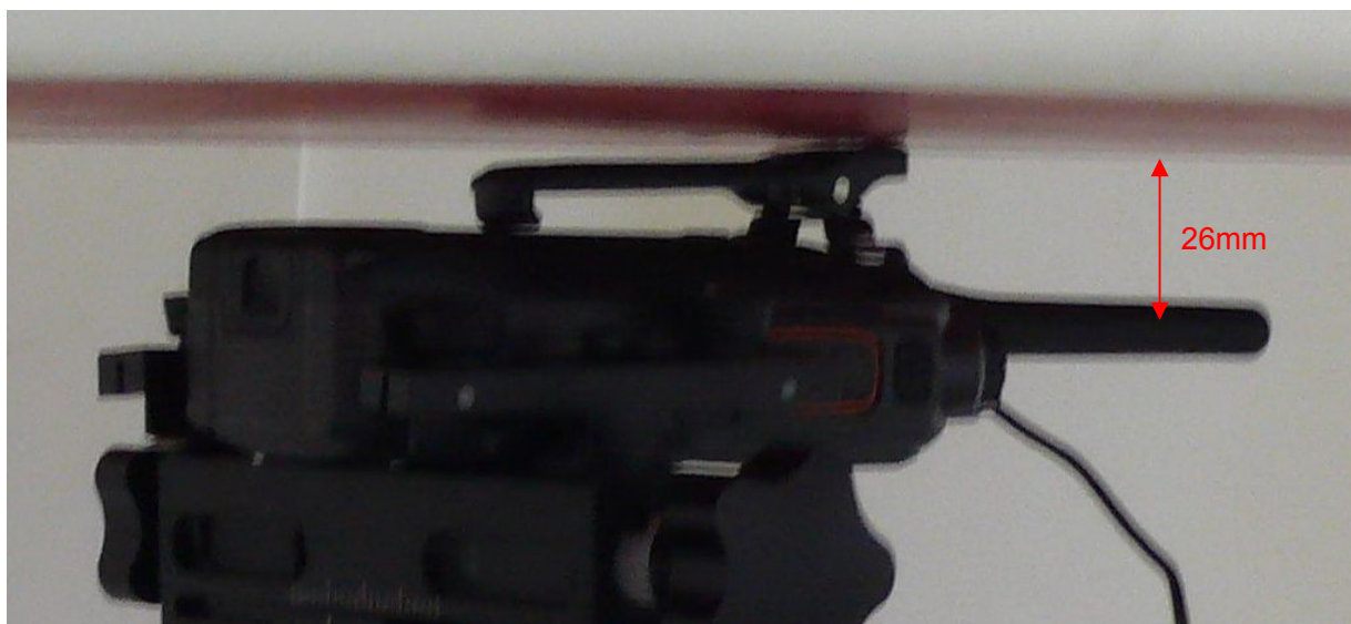
Picture 9: Body-worn with Thinner Battery, Belt and Audio Accessory 2, the front of the EUT towards ground, the distance from EUT Antenna to the bottom of the Phantom is 26mm
