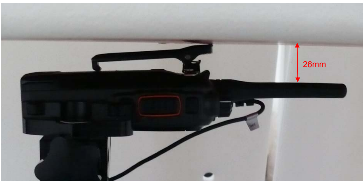
Picture 11: Body-worn with Thinner Battery, Belt and Audio Accessory 4, the front of the EUT towards ground, the distance from EUT Antenna to the bottom of the Phantom is 26mm
