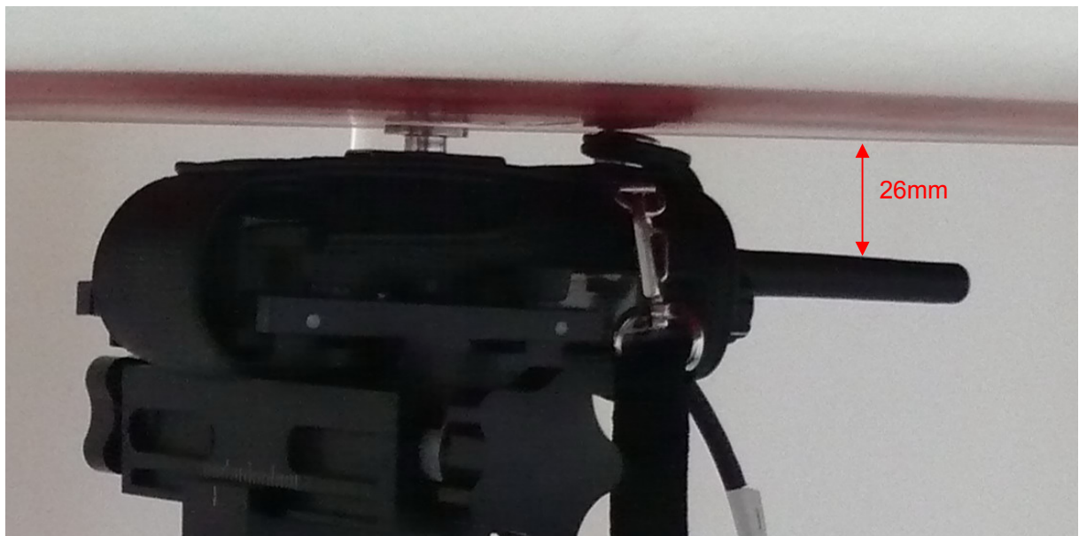
Picture 13: Body-worn with Thinner Battery, Pocket and Accessory 1, the front of the EUT towards ground, the distance from EUT Antenna to the bottom of the Phantom is 26mm
