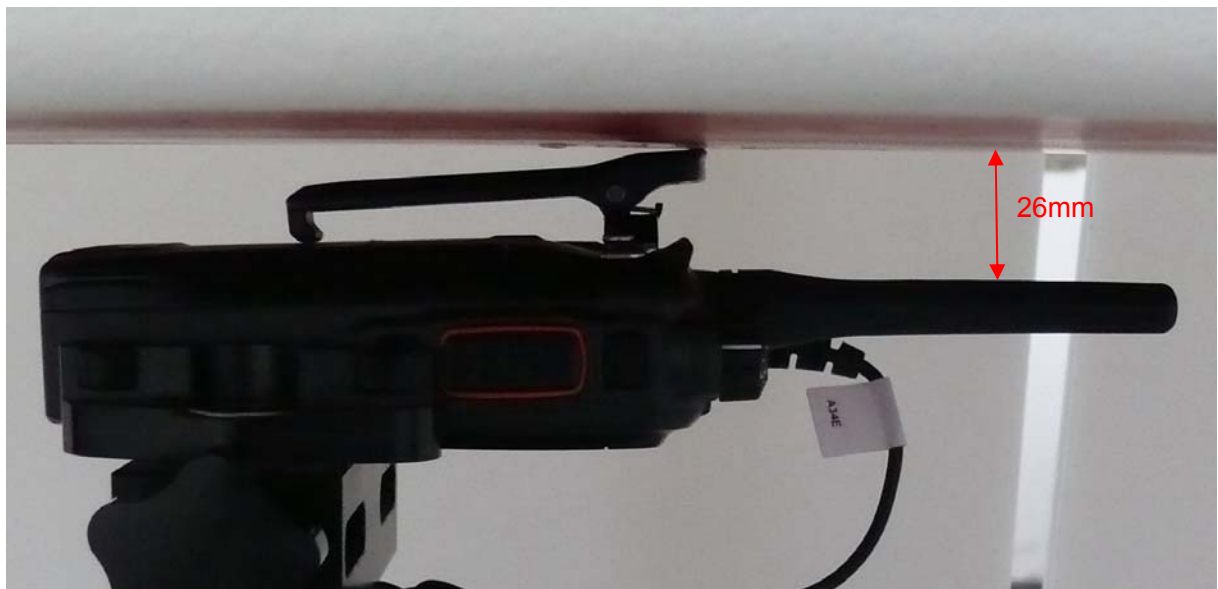
Picture 12: Body-worn with Thinner Battery, Belt and Audio Accessory 5, the front of the EUT towards ground, the distance from EUT Antenna to the bottom of the Phantom is 26mm
