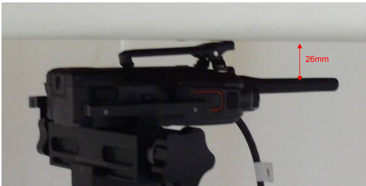
Picture 8: Body-worn with Thinner Battery, Belt, Accessory 1 and Earphone 2, the front of the EUT towards ground, the distance from EUT Antenna to the bottom of the Phantom is 26mm
