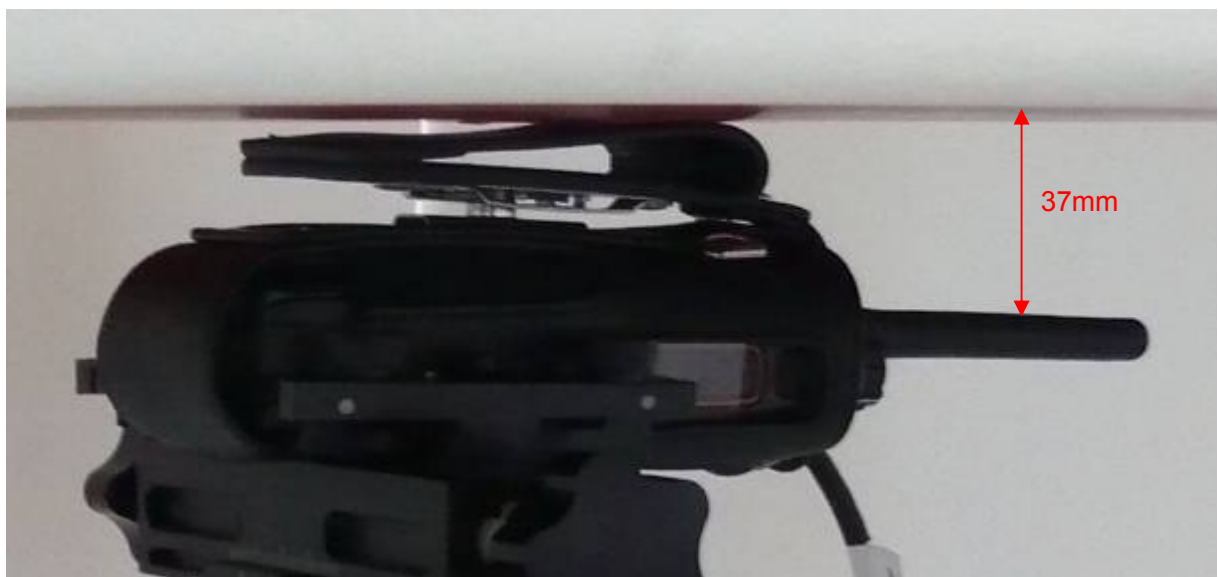
Picture 14: Body-worn with Thinner Battery, Pocket, Leather and Accessory 1, the front of the EUT towards ground, the distance from EUT Antenna to the bottom of the Phantom is 37mm
