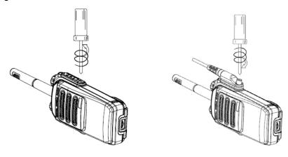
**Step 3** Tighten the screw on the connector.
