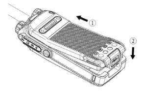
To remove the battery, turn off the radio first. Then slide the battery latch upwards (as 2 shows) to
