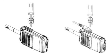
Tighten the screw on the connector.
