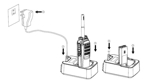
Connect the power adapter to AC socket. See arrow ①.
