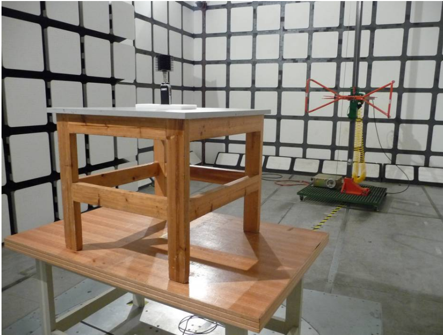
Below 1 GHz: Transmitting Radiated Emissions View
