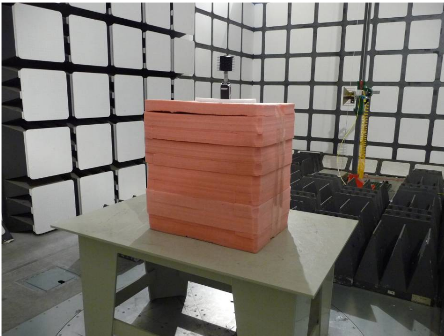
Above 1 GHz: Transmitting Radiated Emissions View
