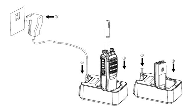
Step 1 Connect the power adapter to AC socket. See arrow 1.
