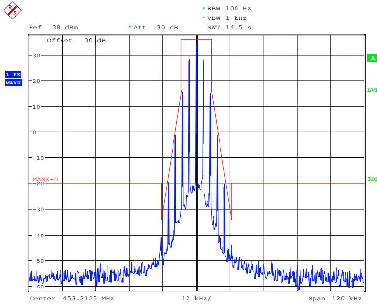
**Frequency 453.2125 MHz: Emission Mask D, Low Power, FCC part 74.462&90.210**
