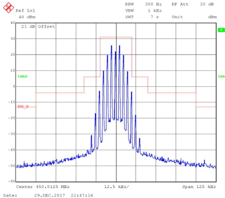
**4FSK,12.5kHz,High Power - Frequency 454.0125 MHz: 99% Occupied & 26 dB Bandwidth**
