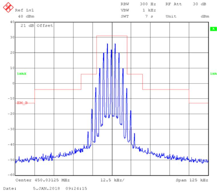
**4FSK,12.5kHz,High Power - Frequency 450.03125 MHz: 99% Occupied & 26 dB Bandwidth**
