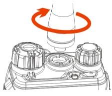
To remove the antenna, rotate it counter-clockwise.
