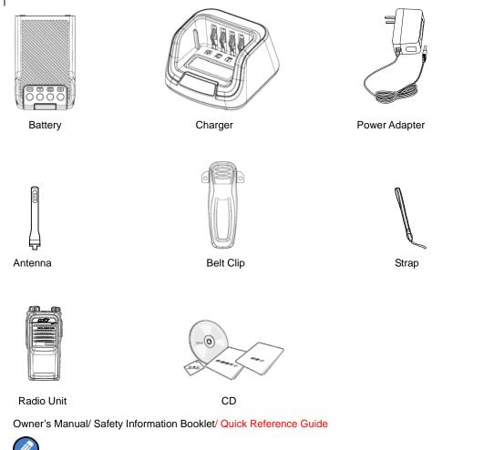
**Note:** The antenna may vary with different frequency bands. And the frequency band is marked on the label of antenna; if not, please refer to the label on the radio unit for frequency band information.
