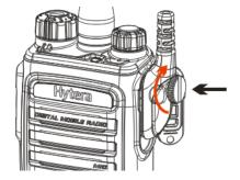
To remove accessories, loosen the screw.
