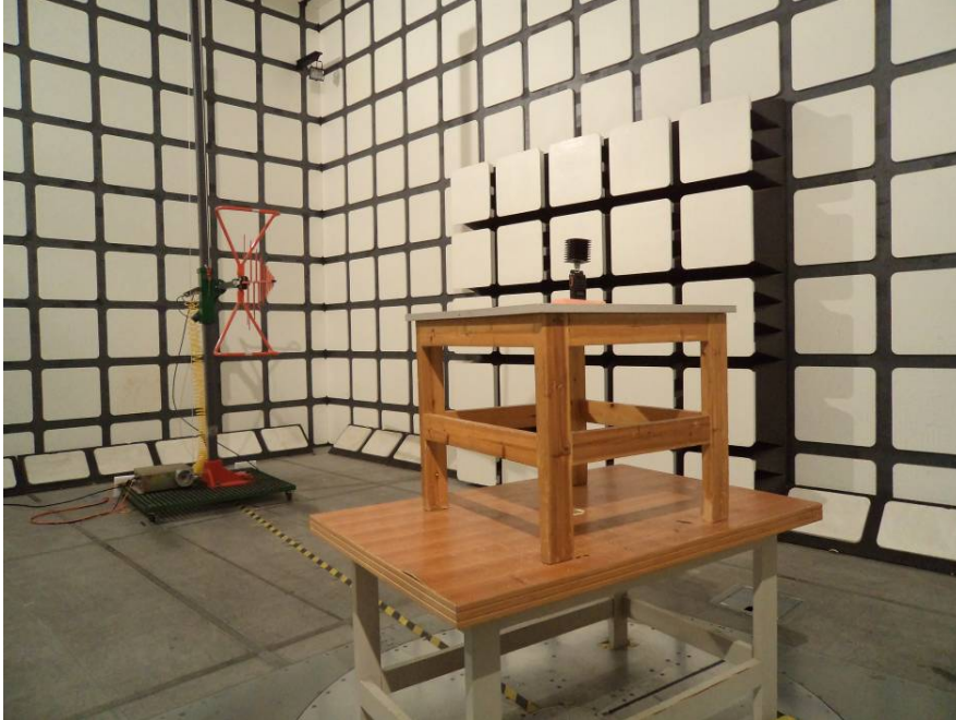
Below 1 GHz: Transmitting Radiated Emissions View
