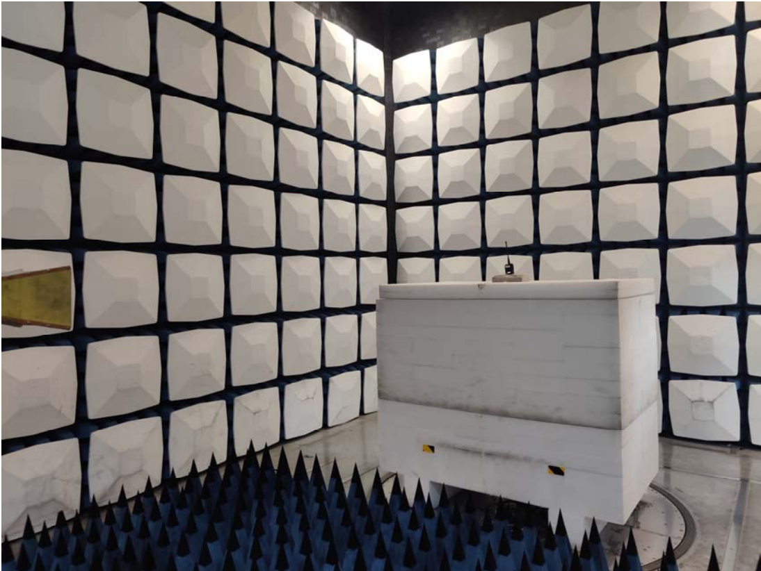
Radiated Emission Above 1GHz View
