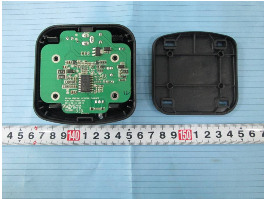
EUT –Charger Cover off View 1
